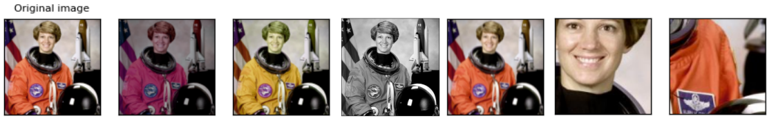
Figure 2.1: Different image transformations applied to the original image. From left to right: original image, color jitter (second and third image), grayscale, Gaussian blur, random cropping (sixth and seventh image). Images are from the documentation of PyTorch.
