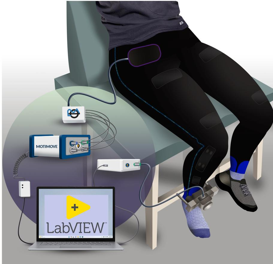
Figure 2.2: Illustration of the experimental setup for the isometric knee extension task using pants embedded with textile electrodes. Details concerning the different components and procedures are provided in the text of the manuscript.
