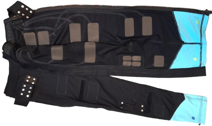
Figure 2.1: Stretchable pants embedded with textile electrodes to stimulate lower limb muscles.
