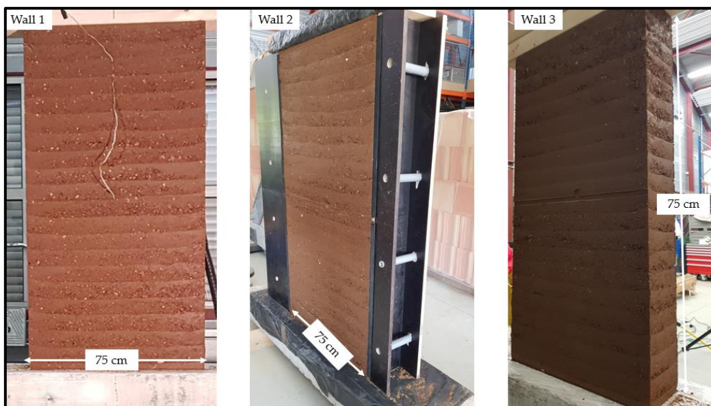
Figure 3.28: Three Rammed earth walls just after manufacture.
