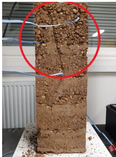
Figure 4.22: A segregation of aggregate during soil mix for samples S12 and S13, causing the upper part of the sample to contain more aggregates while the bottom part is mainly sand and fine.
