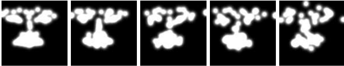
Figure 2.7: Examples of noisy heatmaps. The landmark points were sampled from a gaussian distribution with values of sigma going from 1 to 5 (from left to right).
