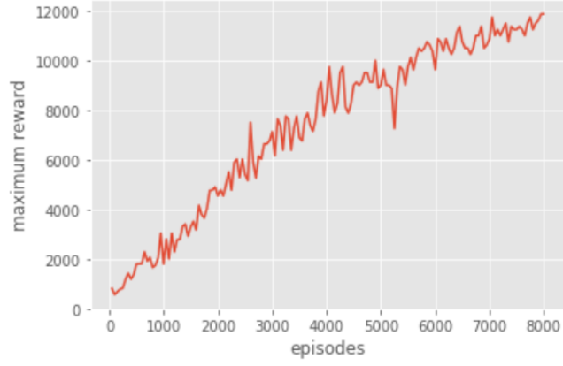
Figure 4.7: The training curves of the mobile node's maximum reward for DQN
