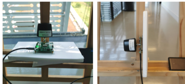
FIGURE 5.12: Two-way ranging with the commercial antenna, characterized by 360^\circ omnidirectional radiation and linear polarization.
