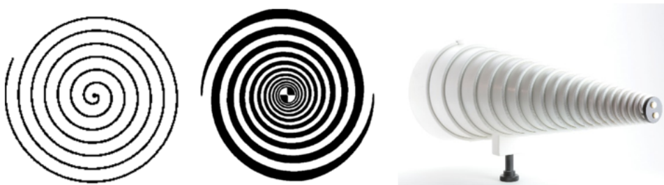
FIGURE 1.12: Antennas defined by angles: Spiral antenna, logarithmic spiral antenna and conical spiral antenna.
