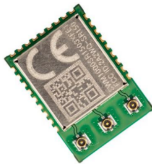
FIGURE 3.12: Sunway Communications' UWB module SR150 interface for ranging and direction finding [19].
