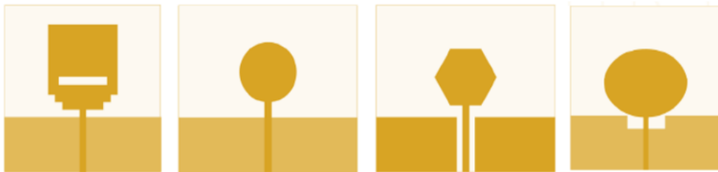
FIGURE 1.16: Planar monopole UWB antennas: two-step band-notch monopole antenna, circular monopole antenna, hexagonal monopole antenna, elliptical monopole antenna with truncated ground plane.
