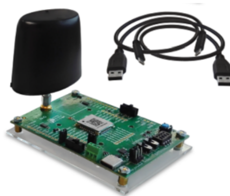
FIGURE 3.10: B-UWB-MEK1 application board for MOD1 module with external antenna [24].
