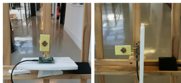
FIGURE 5.13: Two-way ranging with the designed antenna, characterized by 180^\circ directional radiation and circular polarization.
