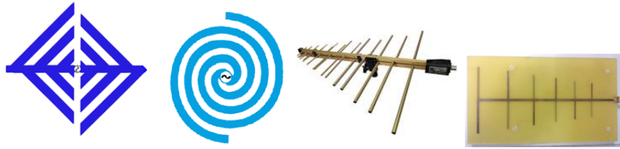
FIGURE 1.11: Two self-complementary antennas of different shapes (rectangular and spiral) and log-periodic antenna in 3D and planar forms.
