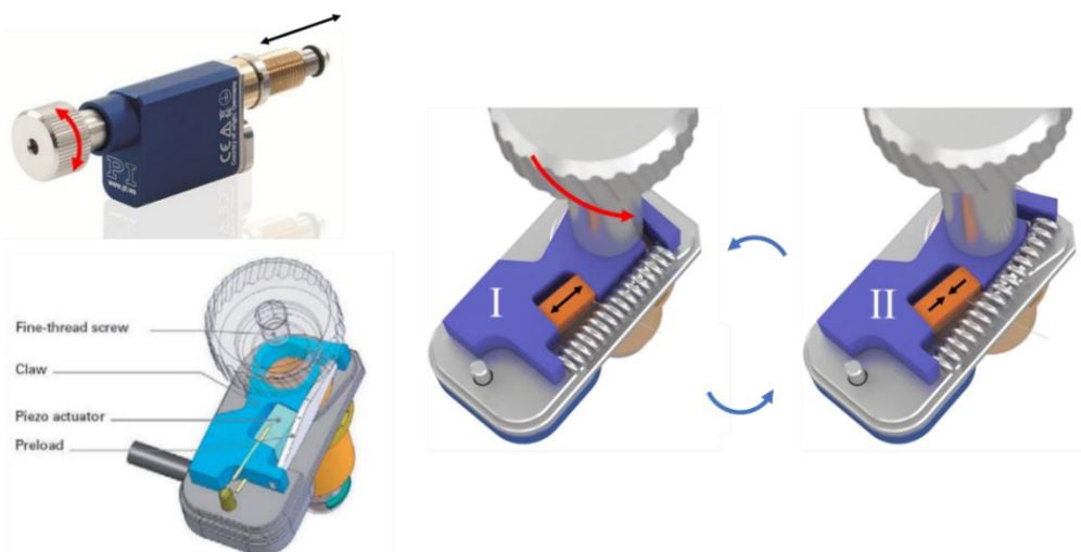
Figure II.8.1-6. PI friction linear motor [47].
