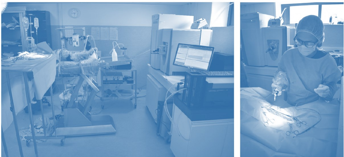
SpiderMass Prototype inside the Oncovet surgery room. Left, General arrangement of the surgery room at the veterinary clinic with the SpiderMass prototype installed beside the surgical table. B. Picture of surgeon with the handled laser microprobe ready to be used during the surgery. Reprinted from Saudemont et al. 1
