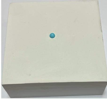
**Figure 2.16:** Picture showing a single rigid PMMA bead, the same as the beads used in the analog fault model shown in Figure 2.1, embedded in a rigid plaster block with dimensions  $10 \times 10 \times \sim 3$  cm.
