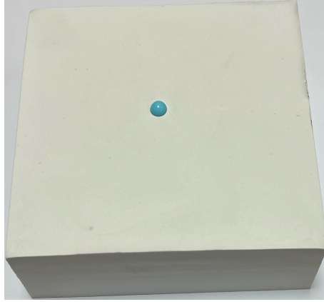
Figure 2.16: Picture showing a single rigid PMMA bead, the same as the beads used in the analog fault model shown in Figure 2.1, embedded in a rigid plaster block with dimensions 10 \times 10 \times \sim 3 cm.
