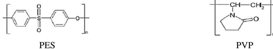
**Figure 1:** Polymers entering in the active layer of the UF membrane
