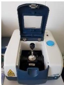
Spectrometer with a membrane coupon
