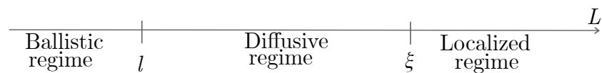
Figure 1.3 – Schematic representation of different transport regimes as a function of the disordered medium length L .
