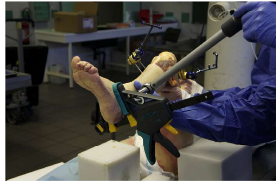
Fig 1. Right lower limb fitted with the navigation system and the torque wrench during tibial internal rotation testing at 90° of knee flexion.
