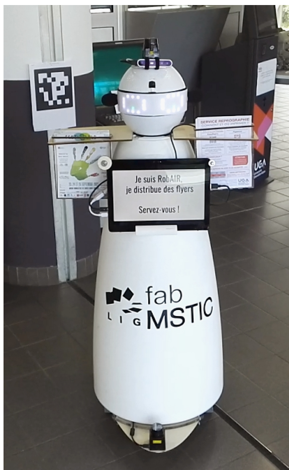
Figure 6.1: RobAIR robot equipped with the flyer holders, and tablet screen UI (translation: "I am RobAIR, I hand out flyers. Help yourself!").
