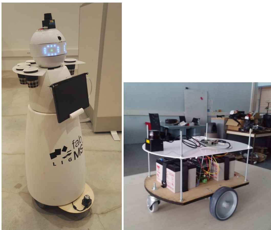
Figure 3.1: Left: RobAIR mobile robot. Right: RobAIR base.
