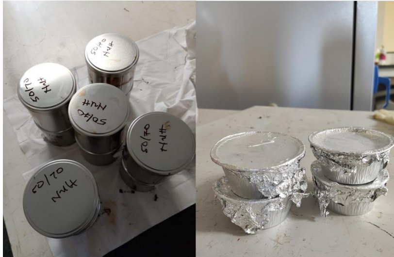
Figure 3.6 – Bitumen proportioned in cans and aluminum cups for storage in the refrigerator
