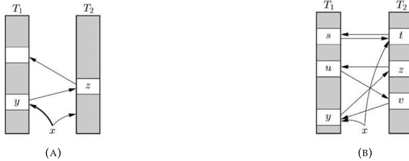
FIGURE 2.1: Cuckoo Hashing insertion examples with two tables. (left) x is inserted with success by moving y and z . (right) x cannot be successfully inserted and a re-hash is required. Figures from (Pagh and Rodler, 2004).
