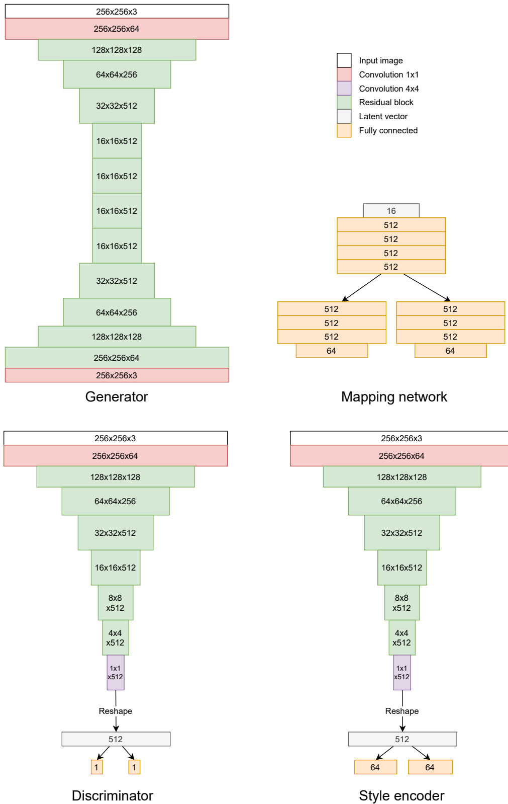
Figure 6.5: The architecture of each sub-network in StarGANv2: Generator (top-left), mapping-network (top-right), discriminator (bottom-left) and style encoder (bottom-right). In this example, the input image is in RGB with the size of 256 \times 256 .
