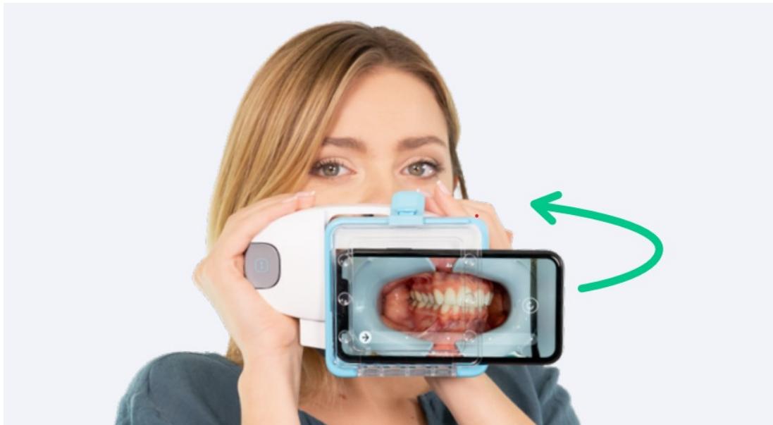
Figure 2.20: A person scanning her teeth using the DM ScanBox. Teeth are closed and the camera is moving horizontally. Image from [31]
