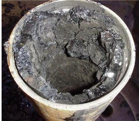
Figure 11. Asphaltene deposition in production tubing in an oilfield in the Gulf of Mexico (reprinted from Borden<sup>47</sup>).
