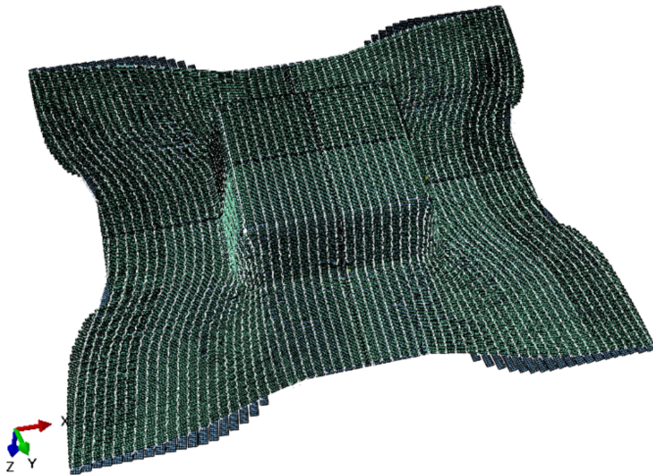
Fig. 4.22: 3D view of square box forming simulation
