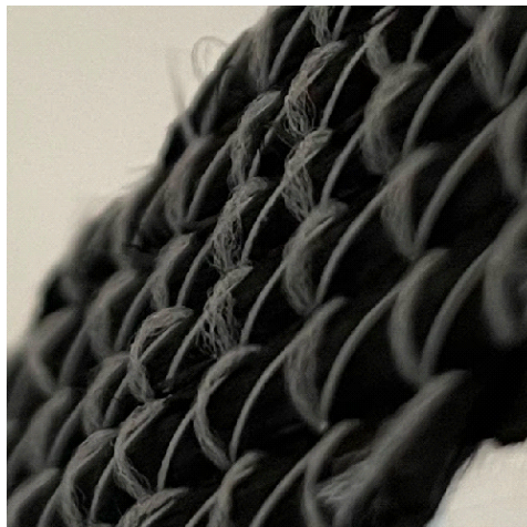
Fig. 2.20: Bent stitch during the shear deformation of bi-axial NCF
