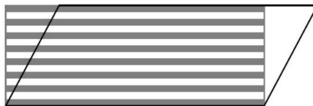
Fig. 1.15: Longitudinal shear of yarn [10]
