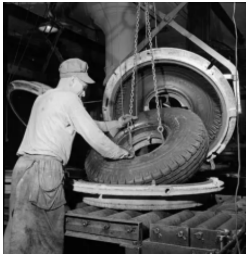
Figure 1.2: Worker removing a tire from an industrial oven used for vulcanization and molding in 1943 (from Flickr, BiblioArchives/LibraryArchives)
