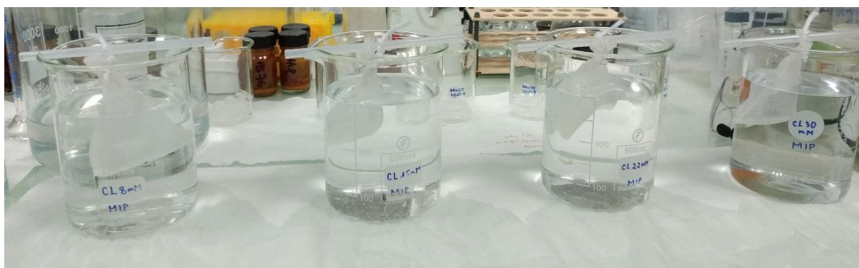
Figure II.3. Tea bags during swelling tests.
