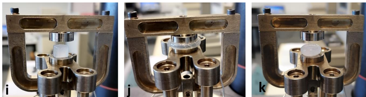
Figure IV.13. Comparison of the behavior of polyacrylamide gels under uniaxial compression (before compressing, under 80% compressing, and after unloading) HG-MBA-0.40 (a, b), HG-MBA-0.75 (c, d), HG-K-MBA-0.40 (e, f), HG-K-MBA-0.75 (g, h) and HG-K-DAEE-Am (i, j, k).
