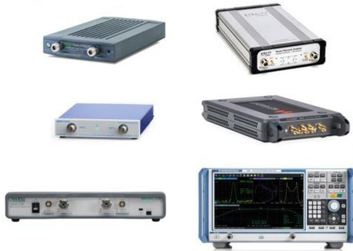
Figure 19. Different existing types and models of the VNA [179]
