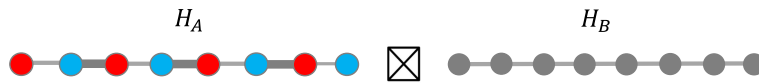
Figure 1.16: Tensor product structure which generates the model illustrated in figure 1.14 a) The left model, given by H_A is a topological SSH models. The right model, given by H_B , is a 1D chain with some on-site and nearest neighbour couplings.
