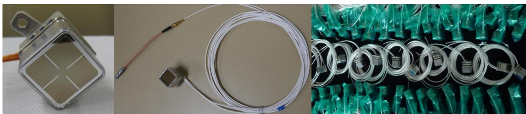
Fig. 2.9 VUV-sensitive Hamamatsu R7600-06MOD-ASSY PMT used in XEMIS2.
