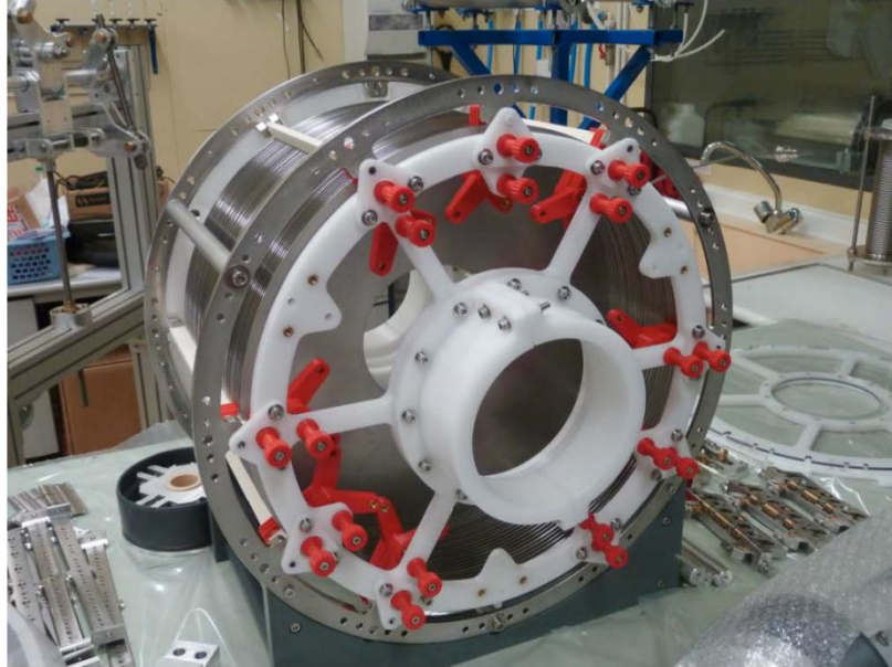
Fig. 2.11 Front view of the cathode with the stainless steel field shaping rings.
