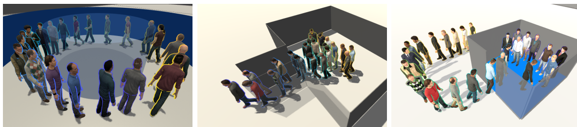
Figure 3.1 – Snapshot of crowd motions generated using the one-man-crowd approach. A single user successively embodies each displayed virtual agent in the order indicated by the highlighting color (from blue to yellow). We studied 3 scenarios that replicated existing experiments from left to right: circular unidirectional flow, bottleneck situation, inflow behavior (entering a lift).
