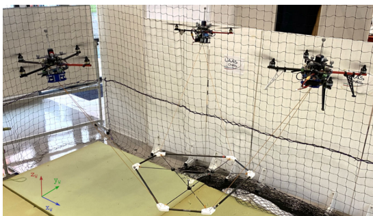
Figure 8.3: [Sanalitra et al., 2022] The Fly-Crane system is a robotic system composed by three aerial vehicles attached to a rigid platform, each one by two cables. This system allows to precisely control both the position and orientation of the platform for aerial manipulation/assembly tasks.
