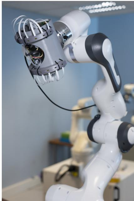
Figure 4.3 – Experimental setup when proximity array is used as an end-effector
