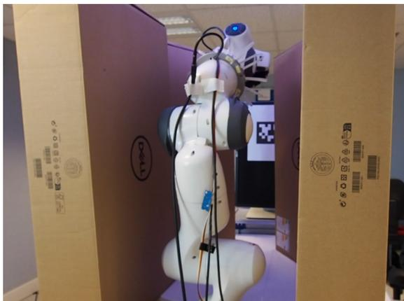
Figure 9.7 – Two blocking planes placed on either side of the robot
