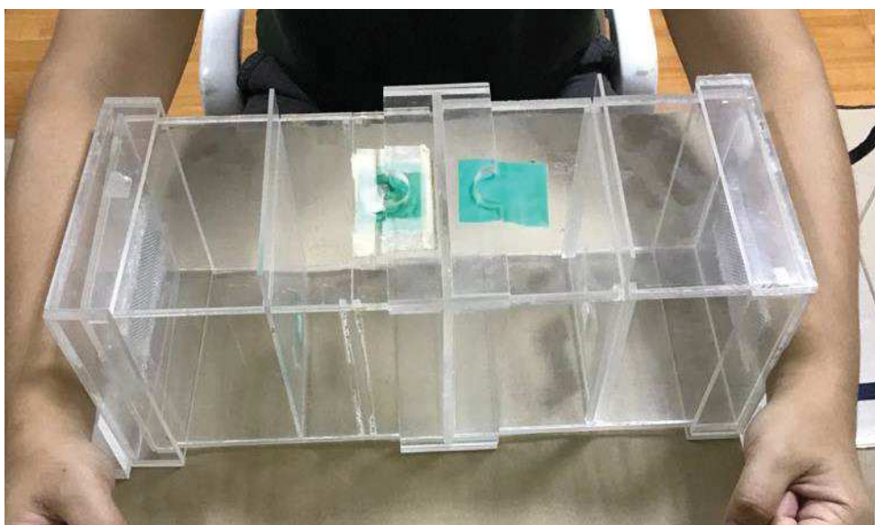
Figure 26 A non-contact repellency assay system (NCRAS) set-up (top view) with volunteer subject sitting in the testing position
