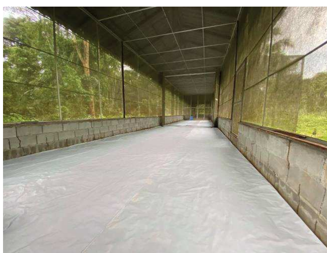
Figure 28 A semi-field screen house (SFSH) measuring 4x3.5x40 m
