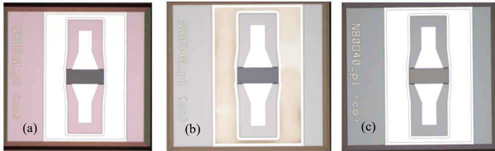
Figure 96: Microscope images after patterning the top electrode for devices with 2.5 \mu\text{m} (a) 3 \mu\text{m} (b) and 4 \mu\text{m} (c) of AlN.
