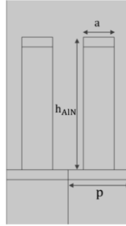
Figure 59: Simplified diagram showing the components of the thickness to pitch ratio and coverage ratio
