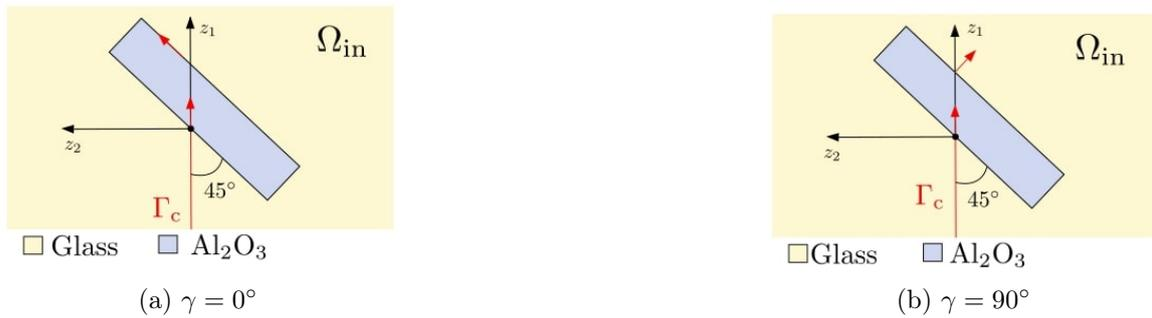
Figure 3.32: Scheme of the inner domain for  $\alpha_p = 45^\circ$  and  $\beta = 45^\circ$  and the expected crack paths (red arrows).
