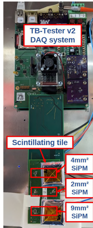
FIGURE 6.14 – Mini-Tileboard with its DAQ system placed in the beam area.
