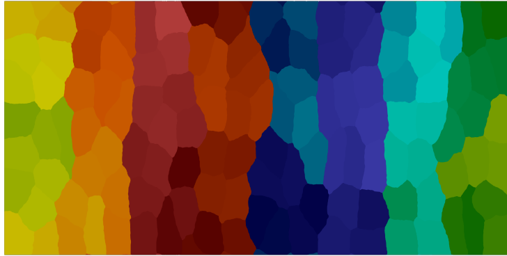
Figure 6.1.10: The decomposition of the 3200 \times 1600 -cell Cartesian mesh into 120 regions where the model is solved in parallel.
