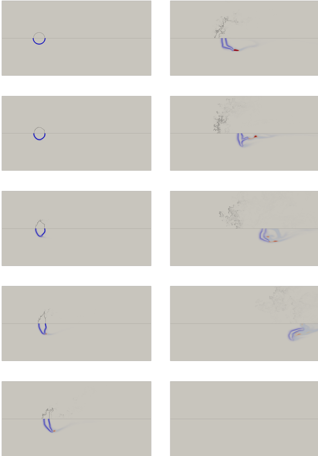
Figure 6.1.16: IAD \|\nabla\alpha_1\| \in (0, 400) \text{ m}^{-1} (top) of the high-fidelity simulation, large-scale IAD \|\nabla\alpha_1\| \in (0, 16) \text{ m}^{-1} (bottom) and small-scale IAD \Sigma \in (0, 34) \text{ m}^{-1} (bottom) of the two-scale simulation. Snapshots are taken each 0.25 s from t = 0 \text{ s} to t = 2.5 \text{ s} from top to bottom and left to right.
