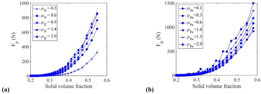
**Figure 3.4** Effects of (a) fiber-fiber friction coefficient  $\mu_{ff}$  and (b) fiber-wall friction coefficient  $\mu_{fw}$  on the loading curves in the uniaxial compression tests (Guo et al., 2021).
