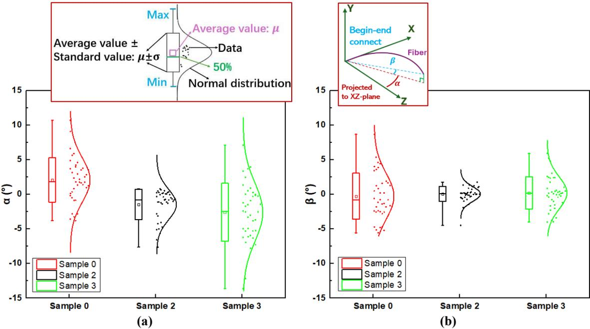
Figure 6.16 The boxplot of mis-orientation angle of fibers for sample 0, 2, 3. (a)  $\alpha$ , (b)  $\beta$  (°).
