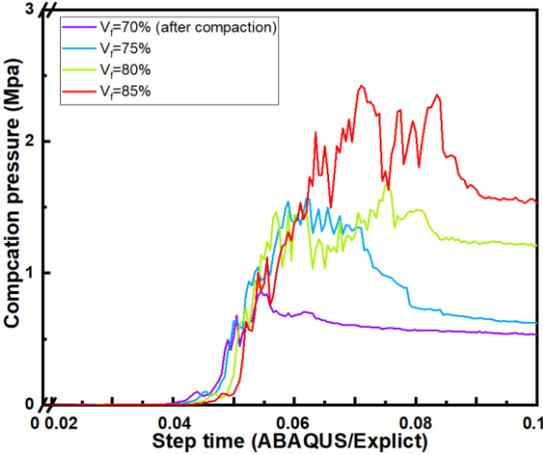
Figure 9.23 Influence of compaction pressure with different compaction states ( $V_f$ ) with relaxation step.
