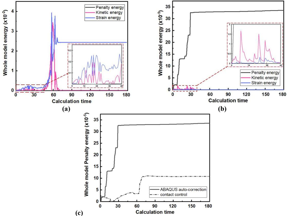
Figure 5.18 The contact, kinetic and strain energy in the initial penetration case with (a) ABAQUS® auto-correction, (b) manually contact control. (c) Penalty energy of this two-method penetration correction.
