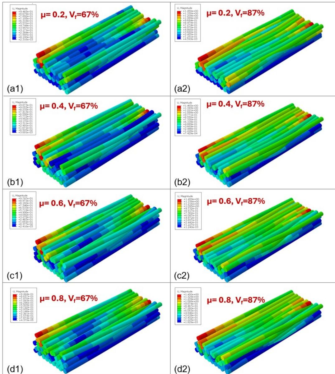
Figure 8.33 3D rendering of fiber bundle geometry with different friction coefficient ( $\mu = 0.2, 0.4, 0.6, 0.8$ ) between fibers, with end volume fraction  $V_f=67\%$  and  $V_f=87\%$ , with compaction performed in Y direction.
