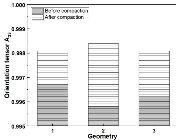
Figure 7.16 Orientation tensor  $A_{33}$  of geometry 1-3 before and after compaction.
