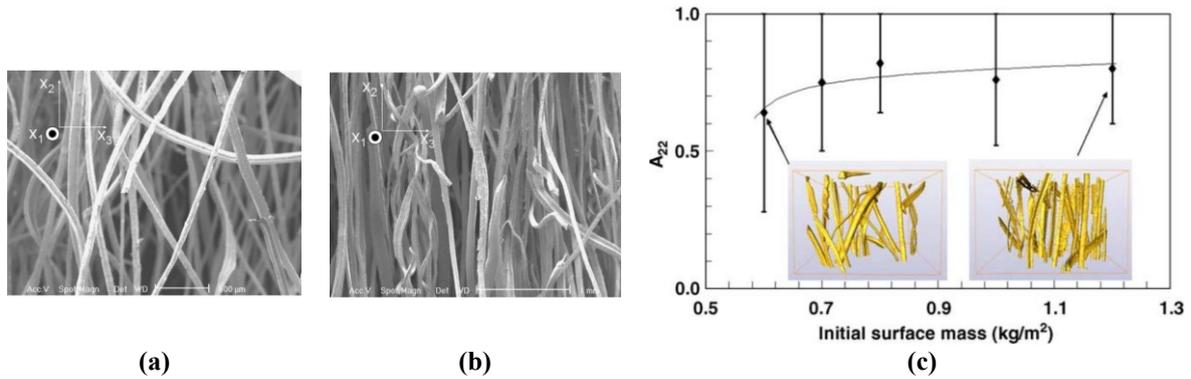
Figure 2.8 The relationship between initial state of fiber assembly and fiber orientation. SEM view of the metallic wools in the thickness in a band of surface mass: (a)  $0.7$  and (b)  $1.3 \text{ kg/m}^2$ . (c) Influence of surface mass on the component  $A_{22}$  of the orientation tensor of the fibers (Masse et al., 2006).
