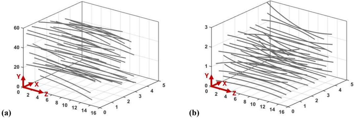
**Figure 7.12 The centerline of fiber bundle geometry 1 created by virtual numerical random fiber bundle generator. (a) Initial fiber bundle (before gravity simulation), (b) After gravity simulation by ABAQUS®.**
