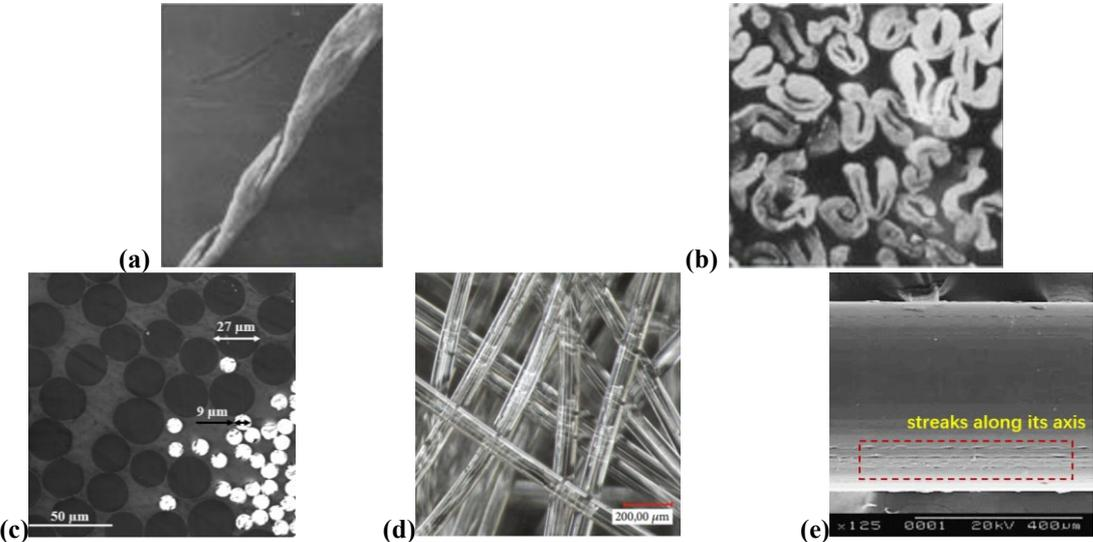
**Figure 1.5 (a) Longitudinal form of cotton fiber. (b) Cross-section form of cotton fiber. (c) Cross-section of polymer fiber (black) and glass fiber (white) (Dalfi et al., 2022). (d, e) Longitudinal form of polymer fiber (Bier et al., 2023; Gassara, 2016).**
