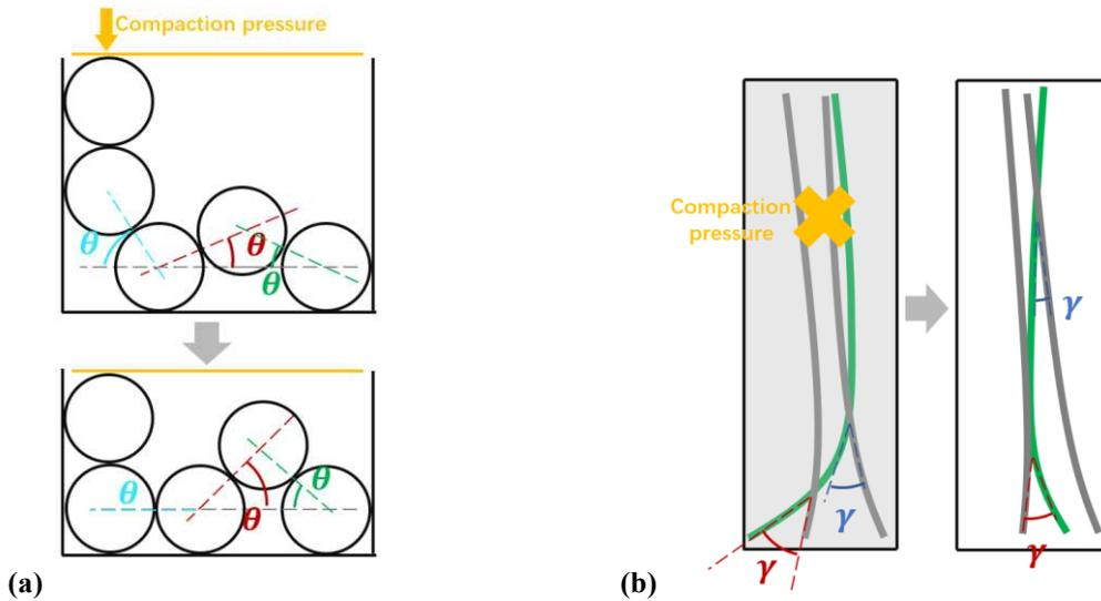
**Figure 6.7 Principle of contact angle in fiber bundle. (a) Contact angle between each two fibers in the section ( $\theta$ ), (b) Contact angle between each two fibers in the fiber length direction ( $\gamma$ ).**
