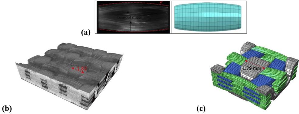
**Figure 2.14 Comparison of the 3D shapes. (a) The yarn, experiment (left), simulation (right) (b) X-ray tomography. (c) with longitudinal compression and transverse extension model (D. Wang et al., 2018).**
