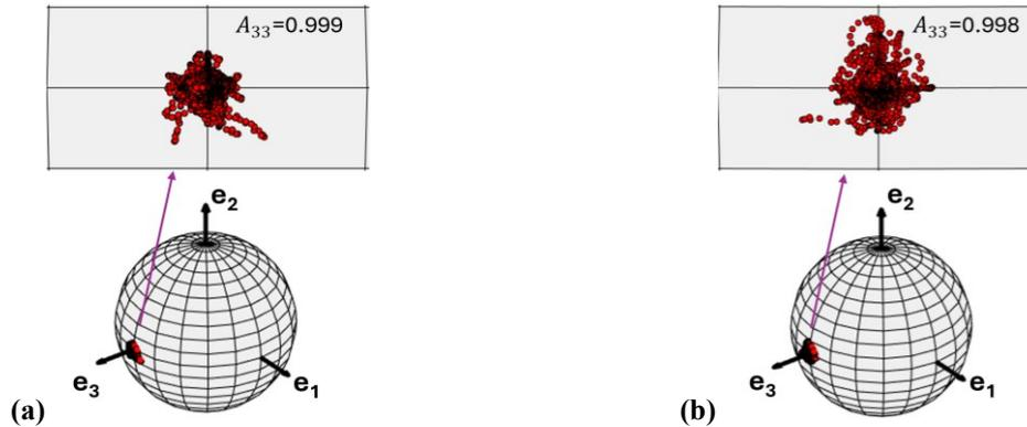
Figure 8.35 Orientation unit spheres of fiber bundle geometry with different  $\mu$  between fibers at  $V_f=87\%$  with X direction compaction. (a)  $\mu=0.2$ , (b)  $\mu=0.8$ .
