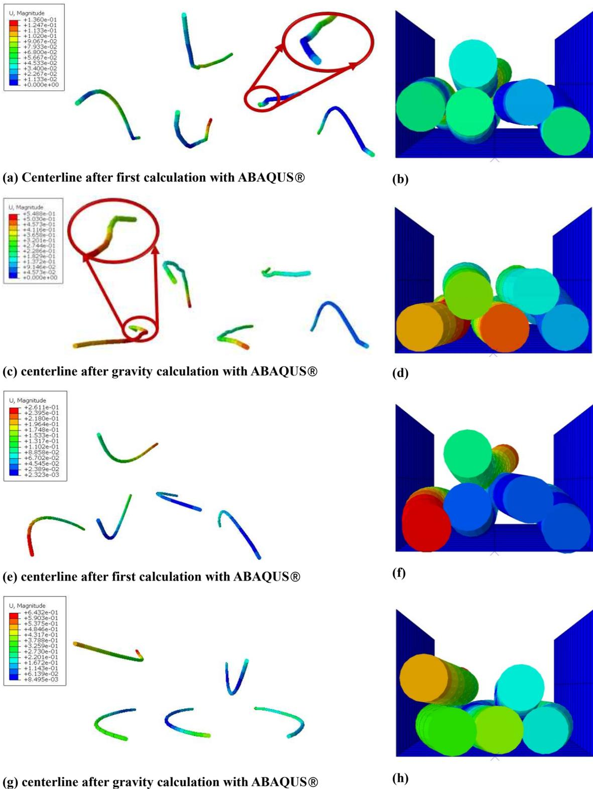
**Figure 5.17 Initial penetration test case. (a, b) after first calculation, (c, d) after gravity calculation with ABAQUS auto-correction; (e, f) after first calculation, (g, h) after gravity calculation with ABAQUS contact control.**
