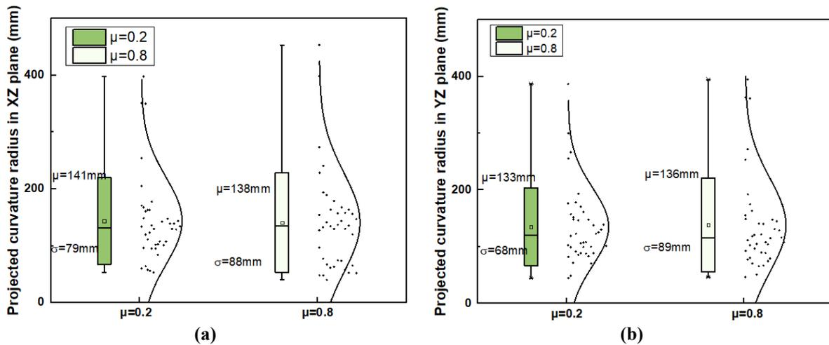
Figure 8.40 Boxplot of projected curvature radii of geometry with  $\mu=0.2$  and  $\mu=0.8$  at  $V_f=87\%$  with X direction compaction. (a) in XZ plane, (b) in YZ plane.
