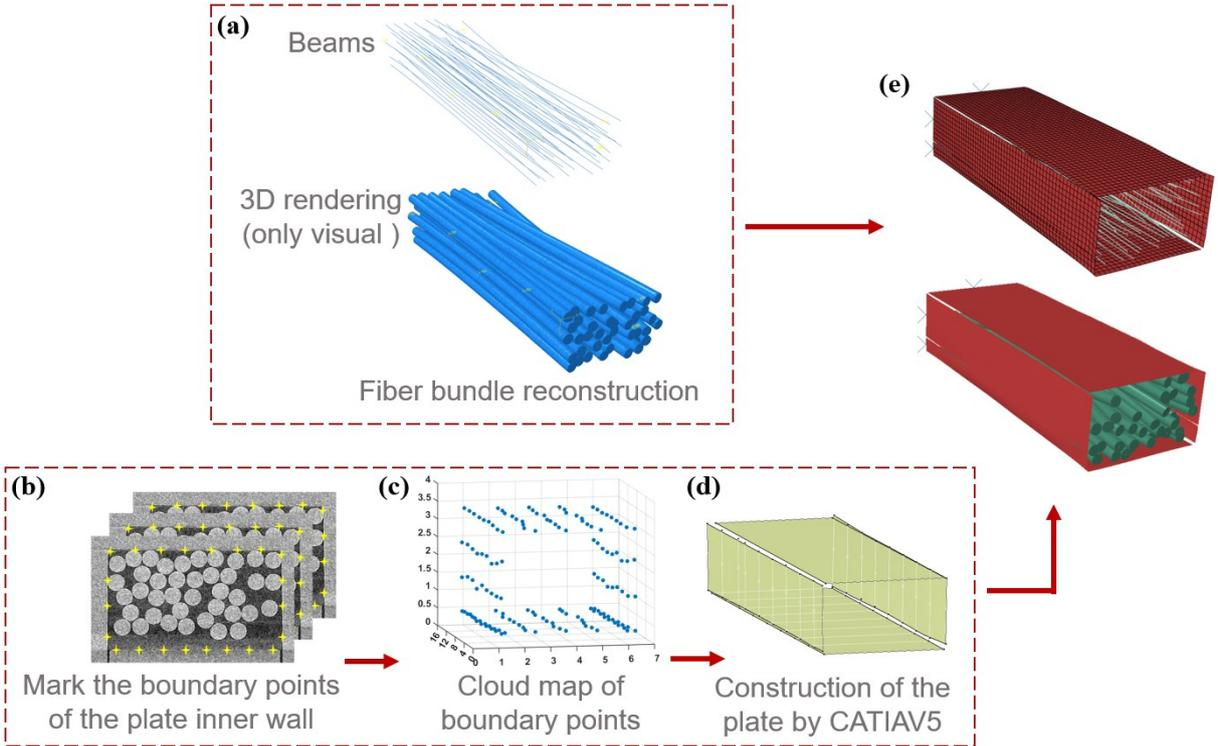
**Figure 5.9** Introduced into the inner wall of the cassette (the compaction channel in contact with the fiber bundle), using Sample 2 as an example: (a) the numerical fiber beams, (b) mark the boundary points of the cassette’s inner wall, (c) the cloud map of the boundary points of (b), (d) construction the compaction channel, (e) import the compaction channel to ABAQUS® with fiber bundle.
