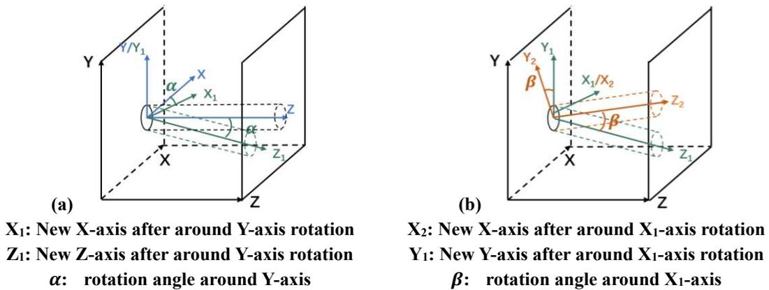
Figure 7.8 Rotation of fibers according to Euler's theory of rotation. (a) Rotation of a single fiber in a separate layer around Y-axis ( $\alpha$ ) ( $^\circ$ ), (b) Rotation of a single fiber in a separate layer around X-axis ( $\beta$ ) ( $^\circ$ ).
