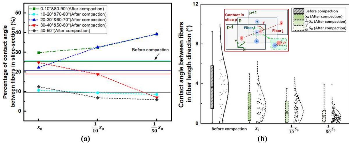
Figure 8.27 Contact angle of geometries with different slenderness ratio of fiber:  $S_0$ ,  $\frac{1}{10}S_0$  and  $\frac{1}{50}S_0$ . (a)  $\theta$  ( $^\circ$ ) in the fiber section, (b)  $\gamma$  ( $^\circ$ ) in the fiber length direction.
