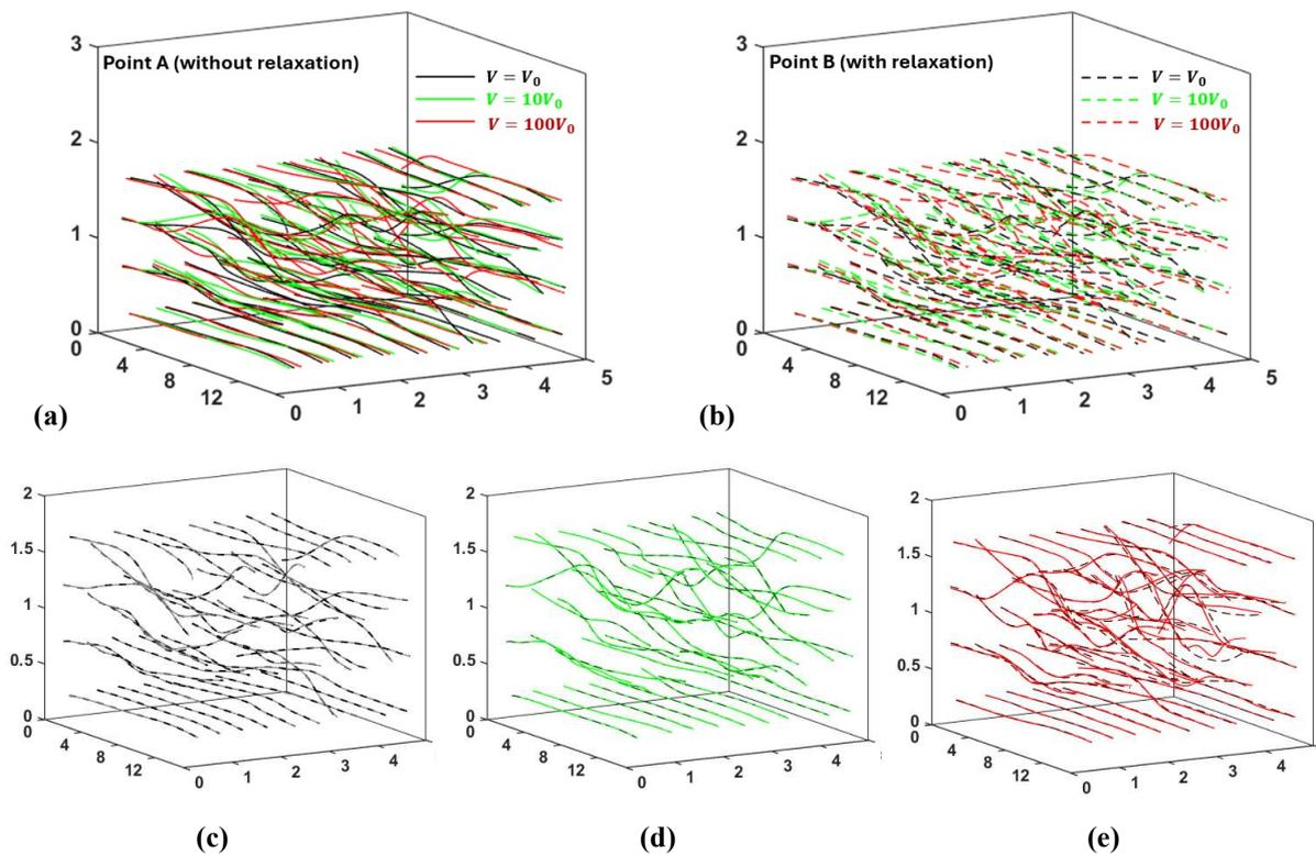
Figure 9.22 Centerline after compaction (a) without relaxation, compaction speed with  $V_0$ ,  $10V_0$ ,  $100V_0$ , (b) with relaxation, compaction speed with  $V_0$ ,  $10V_0$ ,  $100V_0$ , (c) with/without relaxation, compaction speed with  $V_0$ , (d) with/without relaxation, compaction speed with  $10V_0$ , (e) with/without relaxation, compaction speed with  $100V_0$ .
