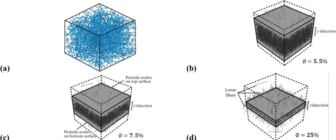
**Figure 3.10 (a) A typical unit cell, containing 692 child fibers. (b-d) Three steps of compaction simulation with 5000 fibers**(A. I. Abd El-Rahman & Tucker, 2013; Ahmed I. Abd El-Rahman & Tucker, 2013).
