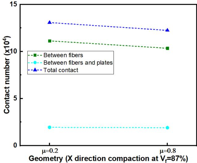
**Figure 8.37 Contact number of fiber bundle geometries with  $\mu=0.2$  and  $\mu=0.8$  at end  $V_f=87\%$  with X direction compaction.**
