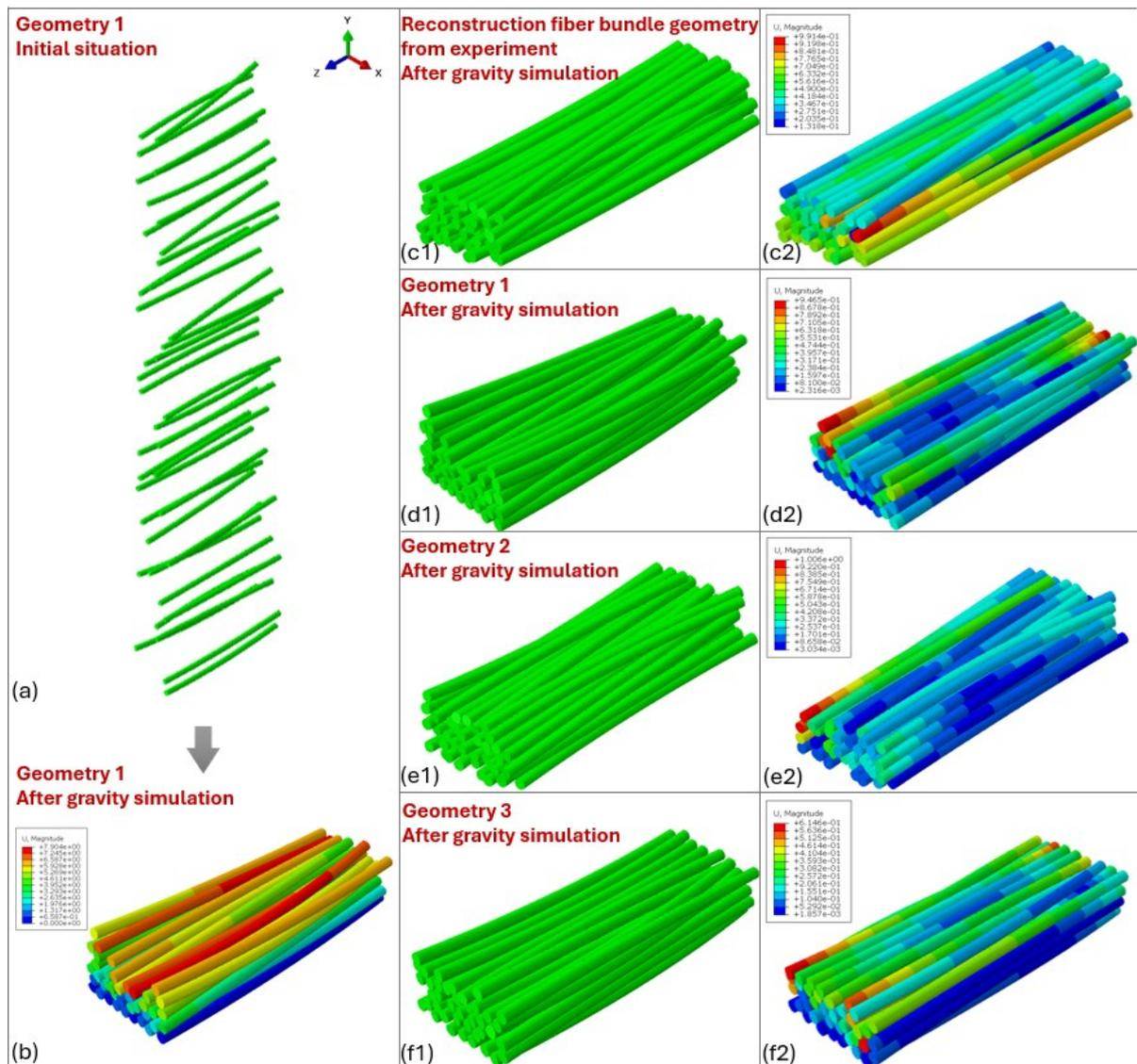
**Figure 7.13 Numerical fiber bundle geometries. (a) The initial geometry 1 before imposing gravity. (b) geometry 1 after ABAQUS® gravity field simulation. (c1) Reconstruction fiber bundle geometry from tomography experiment. (d1-f1) Created geometries after ABAQUS® gravity field simulation, creation parameters same as Sample 2 indicators. (c2-f2) After compaction test with geometries (c1-f1).**
