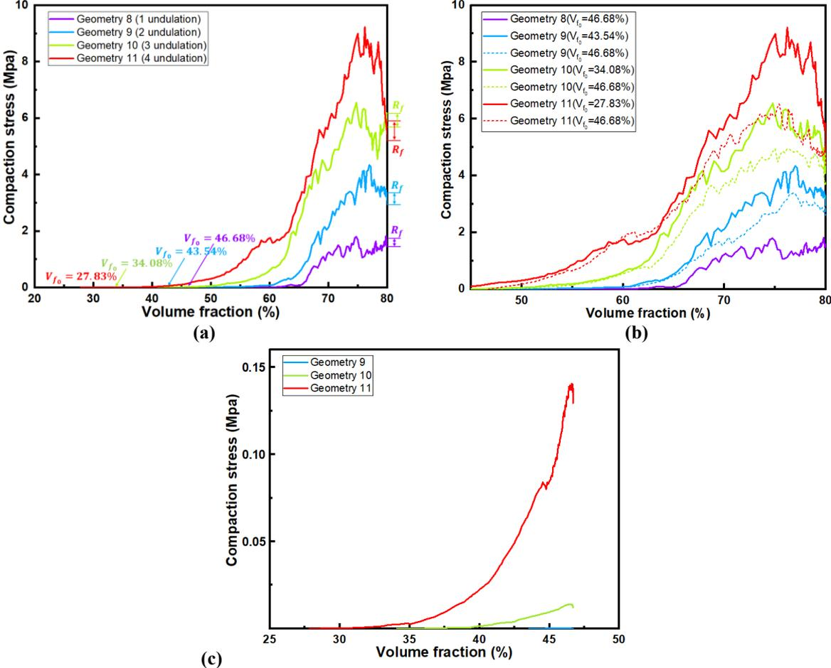
**Figure 8.9 Relationship of Volume Fraction and Compaction Pressure: Geometries 8 to 11, created with different undulation parameters. (a) Compaction test with different  $V_{f0}$ , (b) Compare the compaction test with (a) and (d), (c) Pre-compaction test with different  $V_{f0}$ .**
