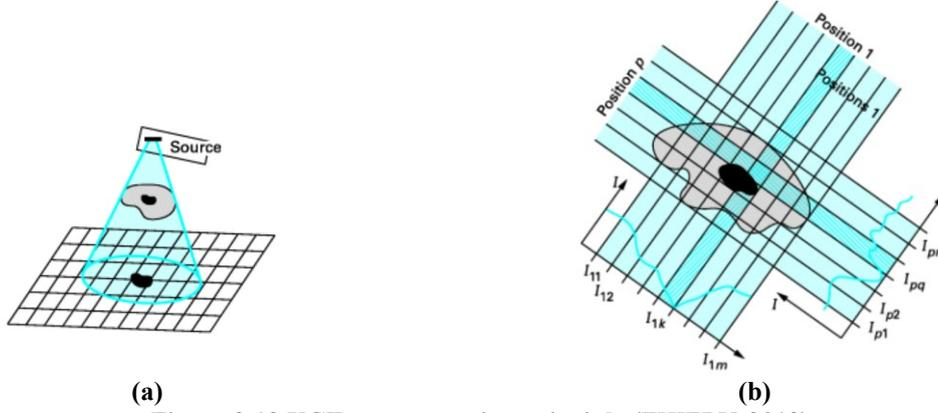
Figure 2.13 XCT reconstruction principle (THIERY, 2013).
