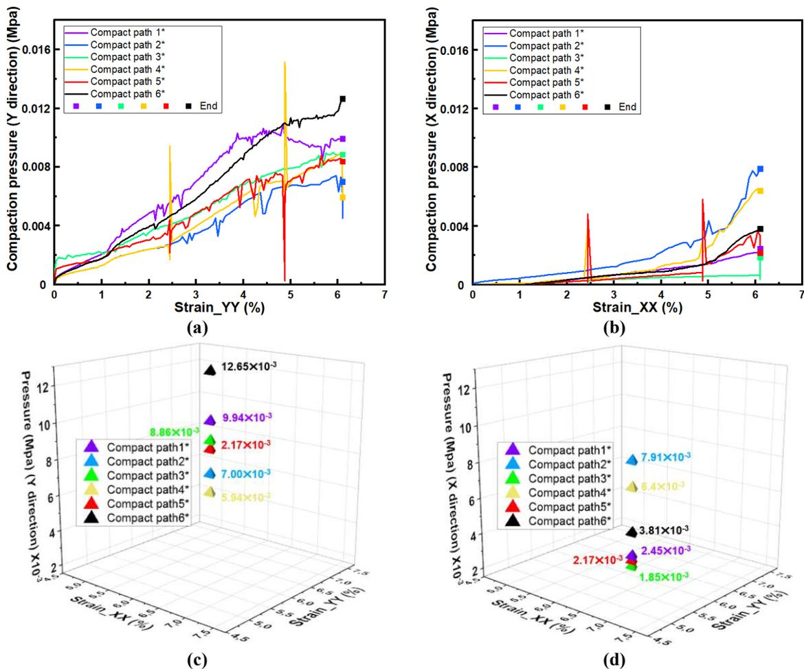
Figure 9.6 Geometry with different compaction path 1\* to 6\*,  $\frac{1}{2} \epsilon_{XX} = \frac{1}{2} \epsilon_{YY} = 6\%$ . (a) Relationship between Strain YY ( $\epsilon_{YY}$ ) and Pressure of Y direction, (b) relationship between Strain XX ( $\epsilon_{XX}$ ) and Pressure of X direction, (c) end of compaction pressure in Y direction, (d) end of compaction pressure in X direction.
