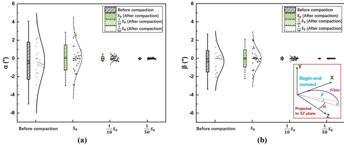
Figure 8.25 Boxplot of mis-orientation of fibers in geometries with different slenderness ratio of fiber:  $S_0$ ,  $\frac{1}{10}S_0$  and  $\frac{1}{50}S_0$ . (a)  $\alpha$  ( $^\circ$ ). (b)  $\beta$  ( $^\circ$ ).
