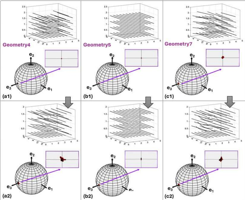
**Figure 8.5 Orientation unit spheres of the centerline of fibers. (a1, b1 and c1) Orientation unit sphere for geometries 4, 5 and 7 before compaction simulation (initial geometry), (a2, b2 and c2) Orientation unit sphere for geometries 4, 5 and 7 after compaction simulation.**
