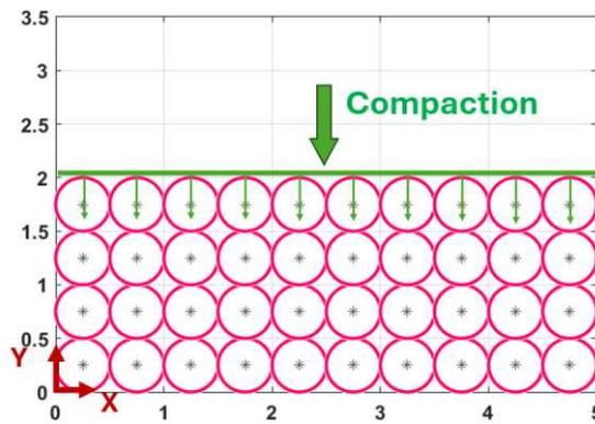
Figure 8.3 Compaction force transfer to fibers of geometry 5.
