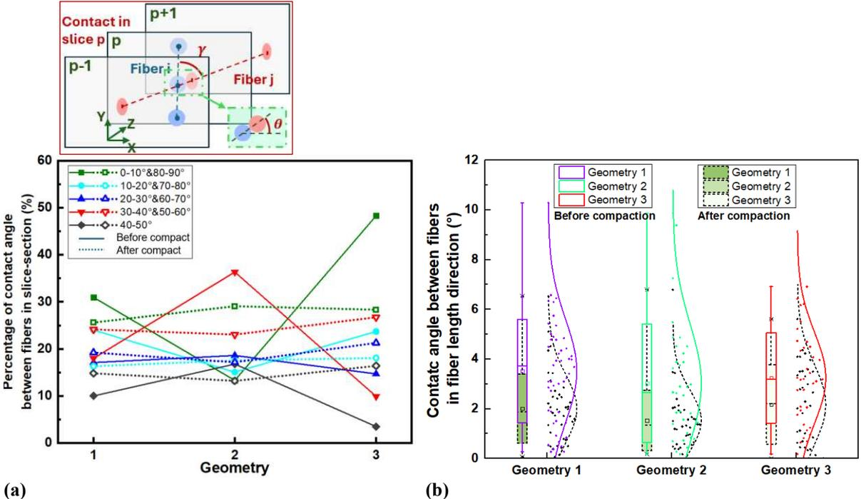
Figure 7.19 Contact angle. (a) Contact angle  $\theta$  ( $^\circ$ ) between fibers in the fiber's section, (b) The boxplot of contact angle  $\gamma$  ( $^\circ$ ) between fibers in the fiber length direction.
