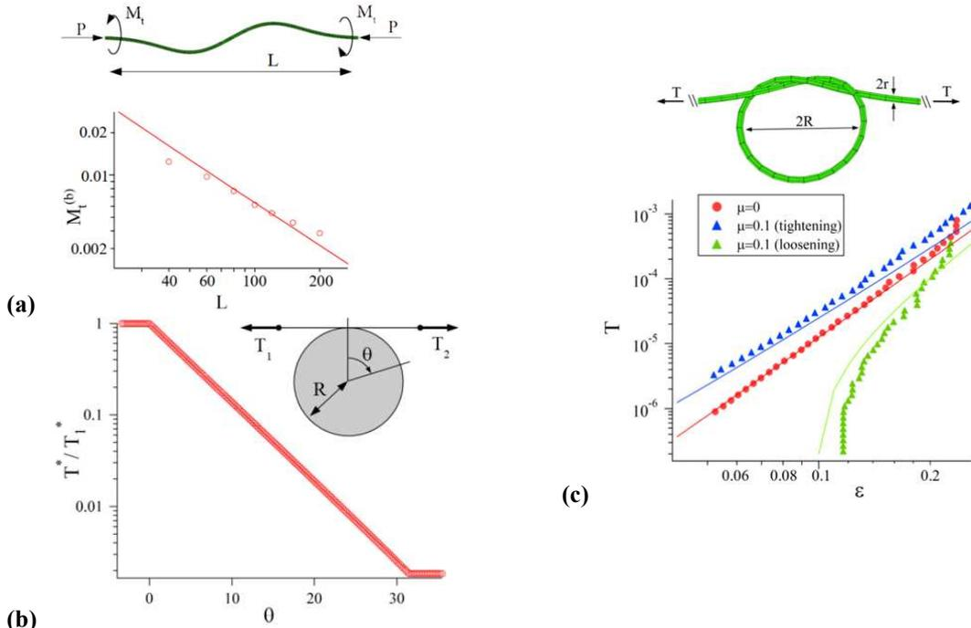
**(a)** Buckling of an elastic rod. Torque applied at ends at the torsional buckling threshold as a function of the rod length. **(b)** Tension in a rolled string around a cylinder:  $T^*$  is the tension in the string, and  $\theta$  is the rolling angle. Circles are symbol, plain line is an exponential fit. **(c)** Tension as a function of  $\varepsilon = \sqrt{r/R}$  for frictionless and frictional strings (Crassous, 2023).
