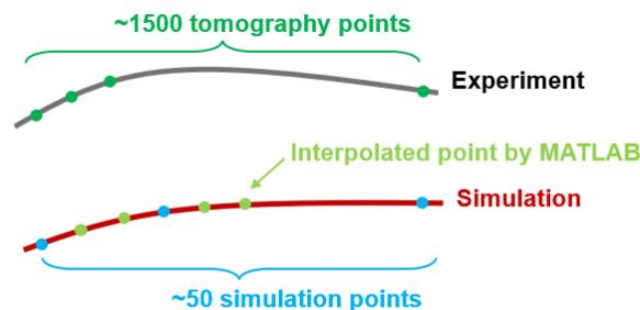
**Figure 6.3 Interpolate points into the simulated fibers.**
