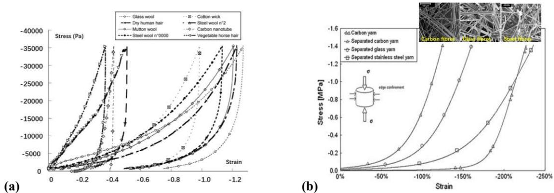
**Figure 2.2** Compression effect of different types of fiber assembly. (a) with same initial density  $150\text{Kg}/\text{m}^3$  (Poquillon et al., 2005). (b) compresses deformation at 6 mm/min (Mezeix et al., 2009).
