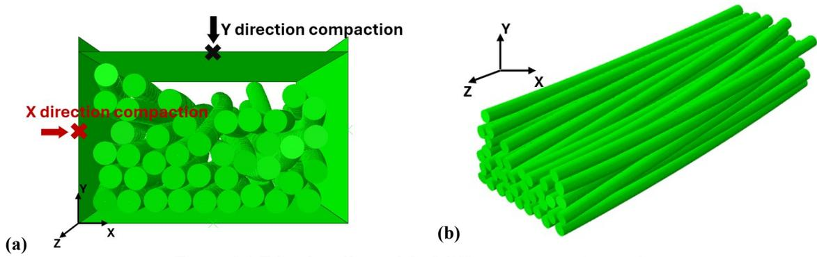
Figure 9.1 Fiber bundle model of different compaction paths.
