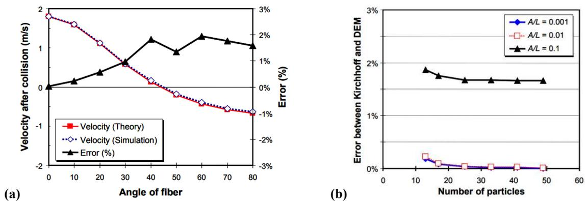
**Figure 3.6 (a) Velocity and error of the rigid fiber after collision. (b) The errors of a vibrating string in frequency with respect to the number of particles when computed by the CFF model ( $A/L$  is a dimensionless proportional parameter used to express the ratio of vibration amplitude to string length.)(Park & Kang, 2009).**
