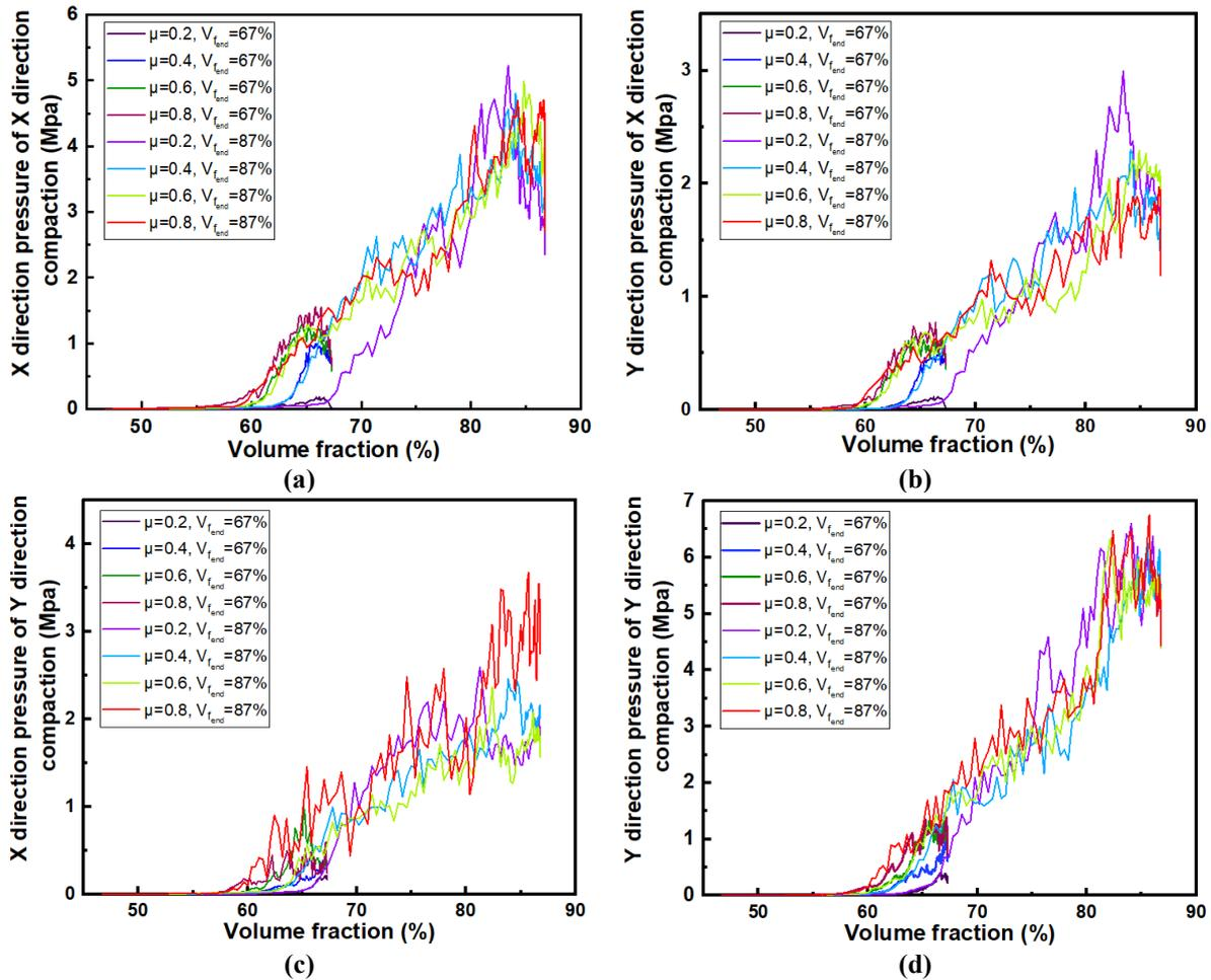
**Figure 8.31 Relationship between volume fraction and compaction pressure of fiber bundle geometry with different friction ( $\mu = 0.2, 0.4, 0.6, 0.8$ ) between fibers, with end volume fraction  $V_f=67\%, 87\%$ . (a) X and (b) Y direction pressure with compaction performed in X direction, (c) X and (d) Y direction pressure with compaction performed in Y direction.**
