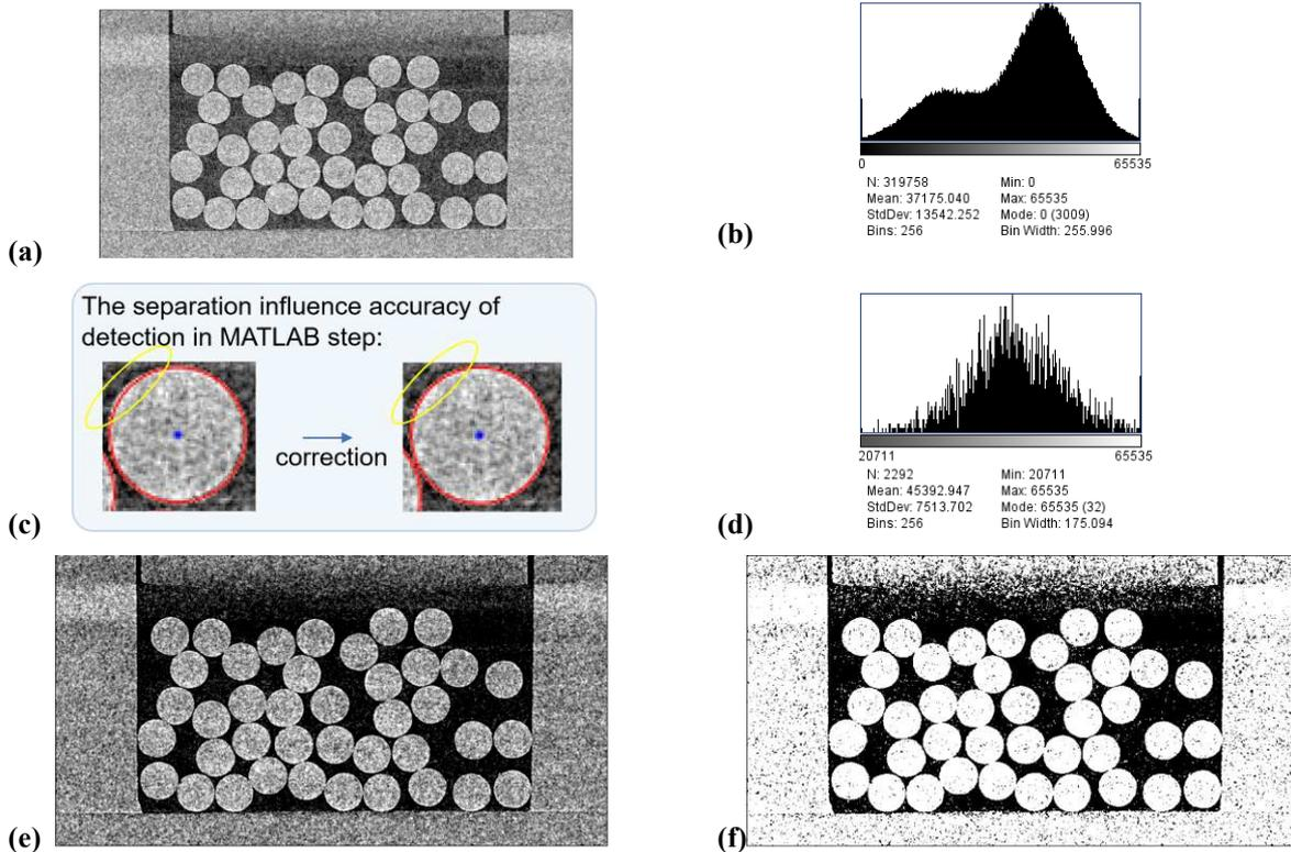
**Figure 5.2** Separation of fibers and voids according to greyscale spectral. (a) Initial slice of fiber's section, (b), (d) the brightness intensity distribution of the slice. (c) The separation influence accuracy of detection in MATLAB step. (e), (f) Different treatment with threshold parameter.
