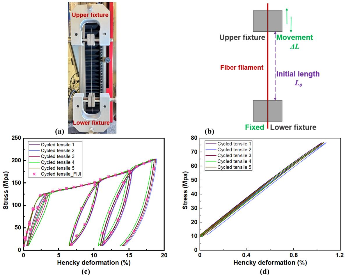
Figure 5.12 Cycled tensile test of polyester fiber. (a, b) tensile machine and principle, (c) 5 cycled tensile test, (d) the first three cycles of the 5 tests.
