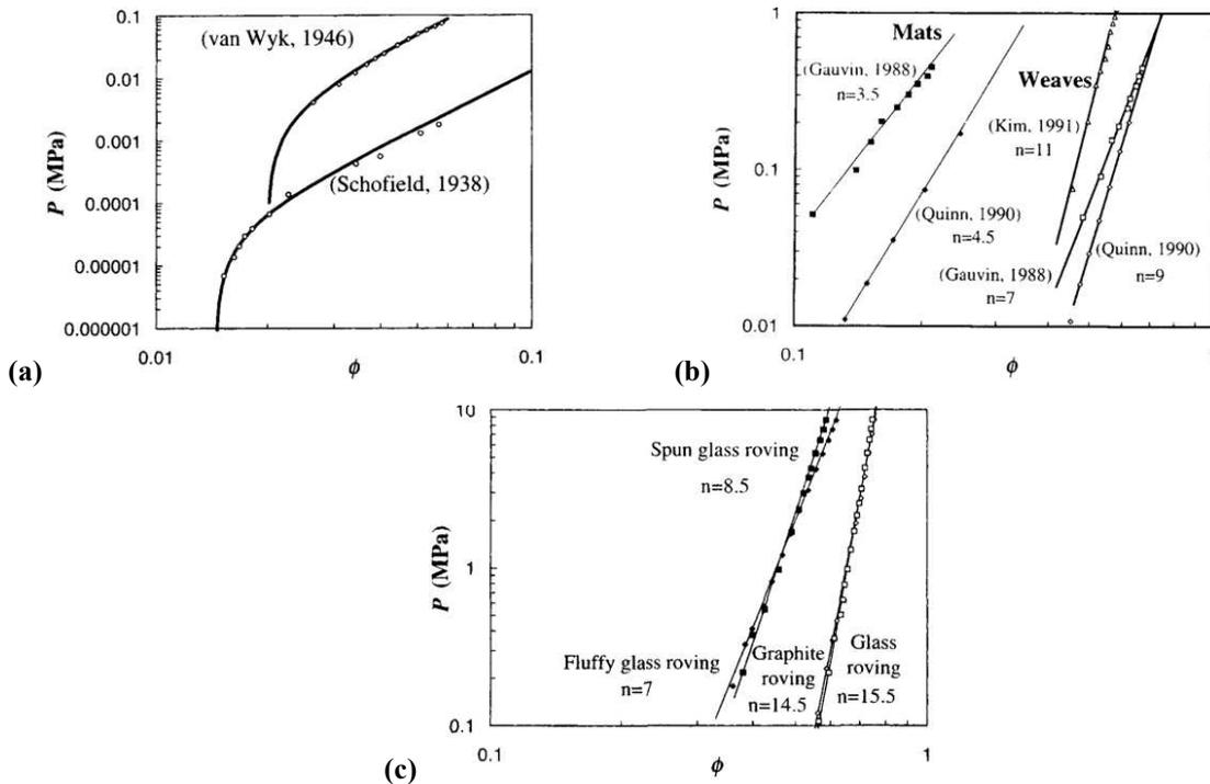
**Figure 2.6** Effect of the morphology for the fiber assembly (a) 3D ( $P = KE(V_f^3 - V_{f_0}^3)$ ), (b) 2D ( $P = KEV_f^n$ ), (c) 1D ( $P = KEV_f^n$ ) (Toll, 1998).
