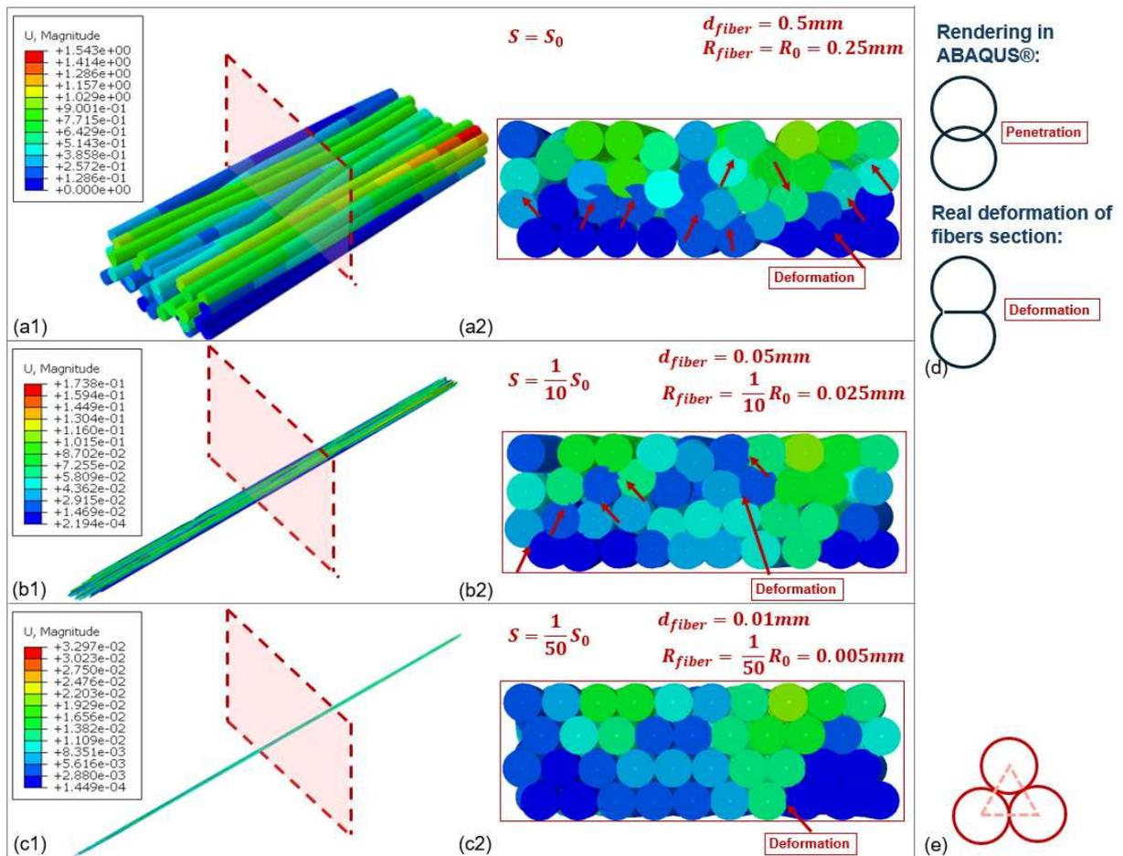
Figure 8.22 Compaction simulations on geometries with different fiber  $S$  ratio. (a1-2)  $S_0$ , (b1-2)  $\frac{1}{10} S_0$ , (c1-2)  $\frac{1}{50} S_0$ , (a-c 1) 3D rendering fiber bundle geometries, (a-c 2) Cross-section of fiber bundle and, (d) principle of contact penetration between fibers with rendering beam and real case of fiber's section deformation, (e) fibers stabilize the triangular structure.
