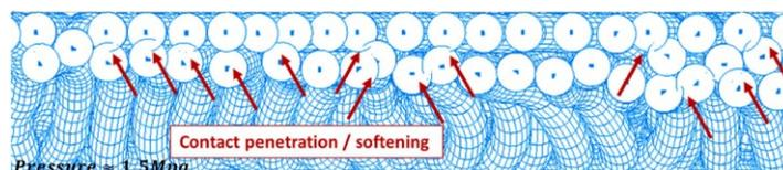
**Figure 3.24 Contact overclosures/penetrations (softening) between neighboring fibers occur in large amounts at pressures 1.5 Mpa (Daelemans et al., 2021).**
