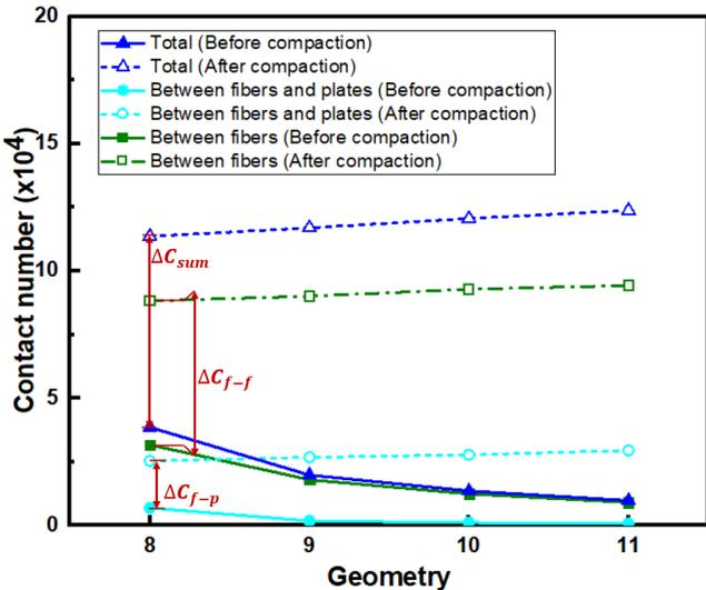
Figure 8.15 Contact number between fibers, fibers and compaction plates and total.
