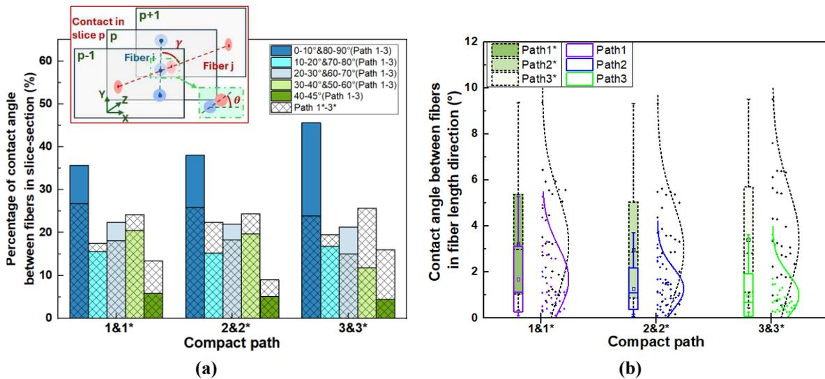
Figure 9.14 Contact angle of compact paths 1 to 3 and 1\* to 3\*. (a)  $\theta$  ( $^\circ$ ) in the fiber section, (b)  $\gamma$  ( $^\circ$ ) in the fiber length direction.
