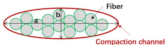
**Figure A The lens-shaped compaction channel.**
