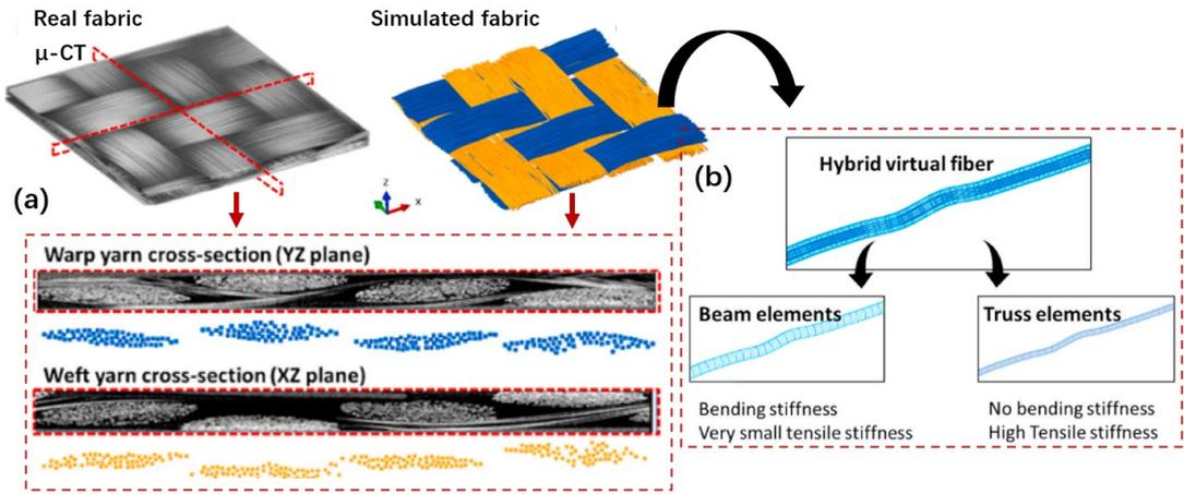
**Figure 3.22 (a) Comparison of real fabric from Micro-CT experiments (left) and simulated fabric (micro-)geometry (right) shows good visual agreement between both. (b) The fabric is constructed of hybrid virtual fibers that consist of a chain of beam elements for bending stiffness and truss element for tensile stiffness (Daelemans et al., 2021).**
