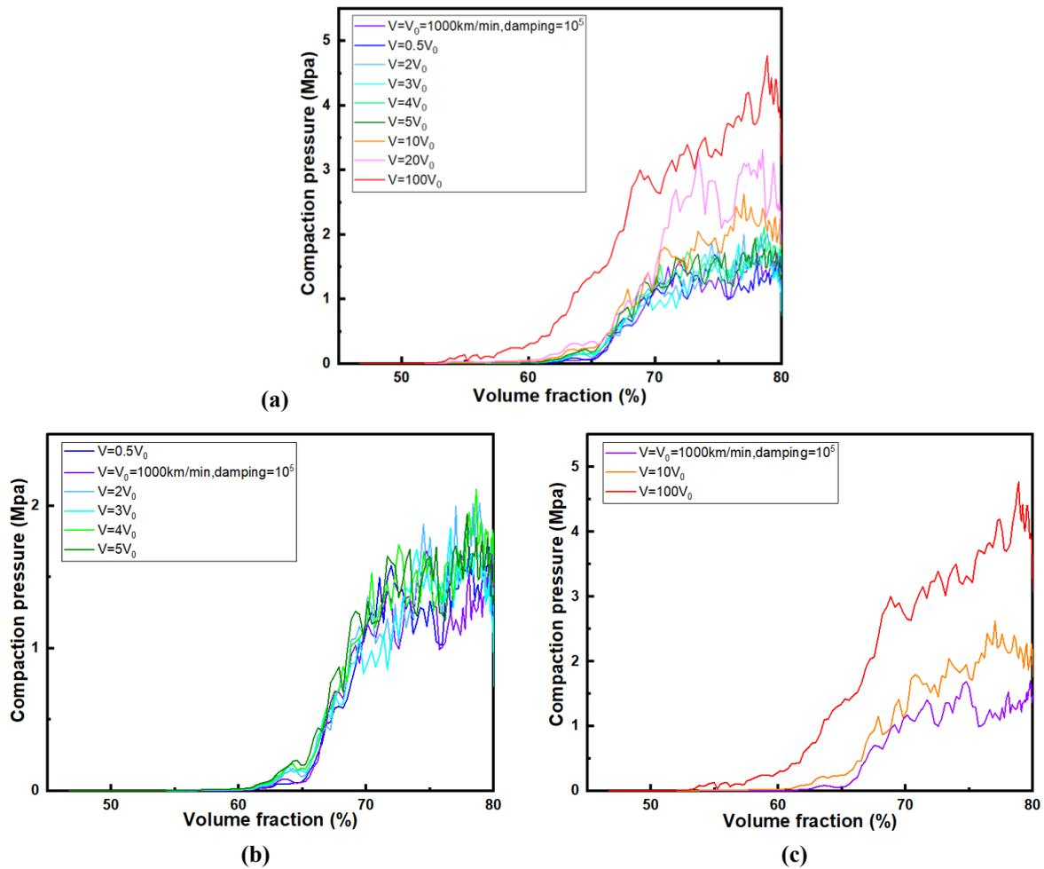
Figure 9.18 Relationship between compaction and volume fraction with different compaction speeds without relaxation step, the reference compaction speed  $V_0=1000$  mm/min with damping coefficient  $\alpha = 10^5$ .
