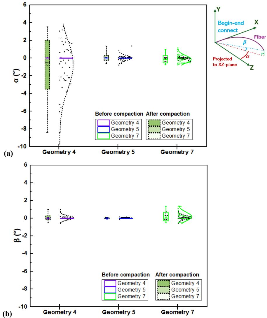
Figure 8.7 Boxplot of mis-orientation of fibers in geometries 4, 5, 7. (a)  $\alpha$  ( $^{\circ}$ ), (b)  $\beta$  ( $^{\circ}$ ).
