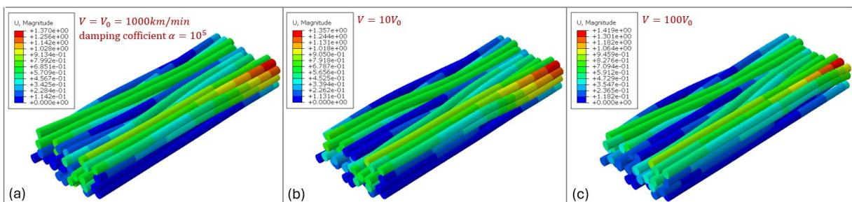
Figure 9.19 3D rendering of geometry after compaction with different compaction speeds without relaxation step, the reference compaction speed  $V_0=1000$  mm/min with damping coefficient  $\alpha = 10^5$ .
