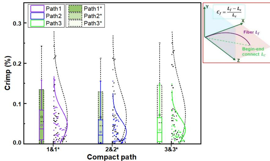
Figure 9.16 Crimp of compaction paths 1 to 3 and 1\* to 3\* (%).
