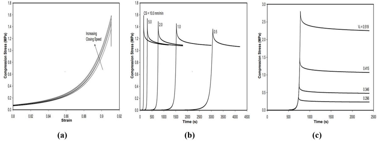
**Figure 2.4 Continuous Filament Random Mat (CFRM) Compaction tests. (a) Compaction speed tests,  $V_f$  (volume fraction at end of compaction) = 0.415. (b) Compaction/relaxation speed tests,  $V_f = 0.415$  (c) Compaction level ( $V_f$ ) tests, CS=2.0mm/min (Arcot Arumugam Somashekar, 2009).**
