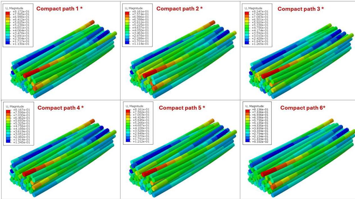
Figure 9.8 Simulation with 6 different compaction path 1\* to 6\*,  $\frac{1}{2} \varepsilon_{XX} = \frac{1}{2} \varepsilon_{YY} = 6\%$ .
