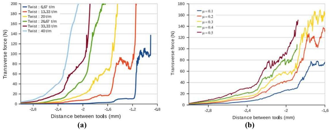
**Figure 3.18** The compression force in function of distance between two compaction plates. (a) with different roving geometry. (b) with different friction coefficient (Moustaghfir et al., 2013).
