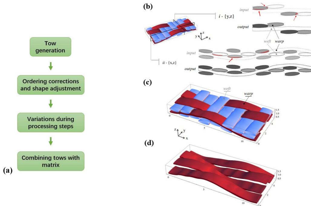
**Figure 3.2 (a) Generation step of 3D virtual fabric. (b-d) Virtual specimen one unit cell in size, defined on a grid with  $N_x=120$  and  $N_y=60$ : (b) Illustration of interpenetration removal on two different cross sections. (c) 3D rendering of the output corrected virtual specimen. (d) 3D rendering of the output warp tows only (Rinaldi et al., 2012).**
