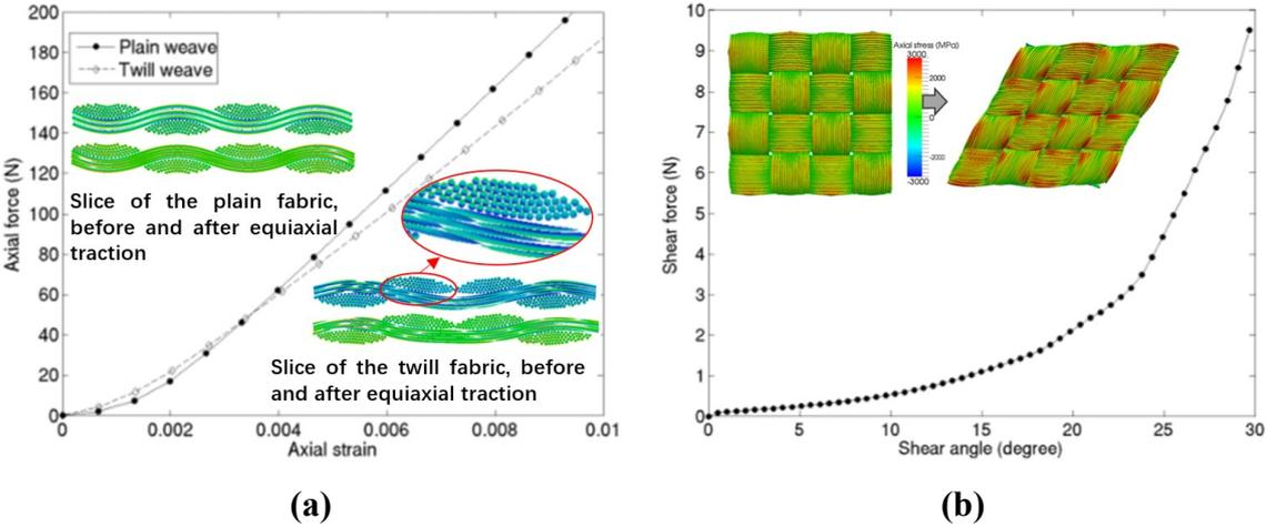
**Figure 3.15 (a)** Simulation of the bi-axial traction of twill and plain weave fabric: axial force as a function of the axial deformation. **(b)** Simulation of shearing of plain weave: shear force as a function of shear angle(D. Durville, 2011).
