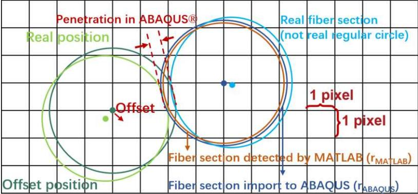
Figure 5.15 Penetration principle between fibers in ABAQUS®.
