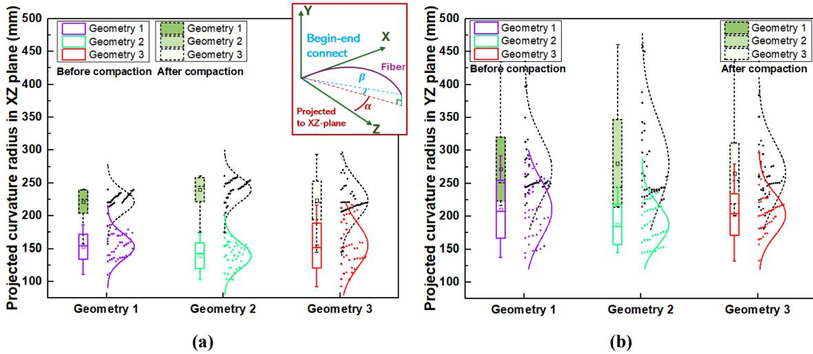
Figure 7.21 The boxplot of projected curvature radii (mm) of fiber bundle geometry 1-3, (a) In XZ plane. (b) In YZ plane.
