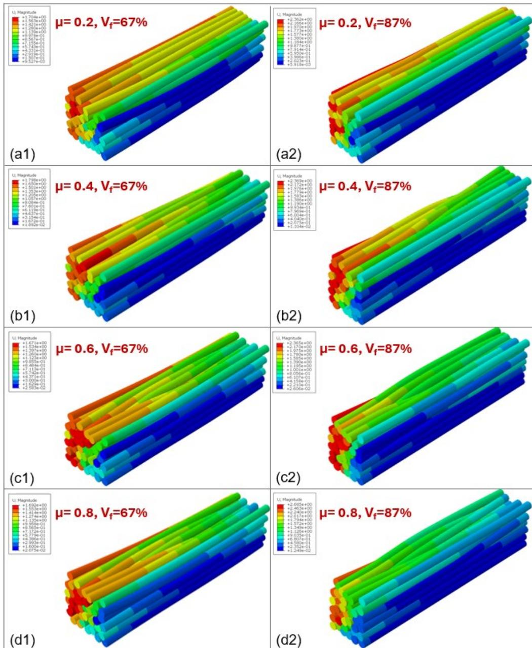
Figure 8.32 3D rendering of fiber bundle geometry with different friction coefficient ( $\mu = 0.2, 0.4, 0.6, 0.8$ ) between fibers, with end volume fraction  $V_f=67\%$  and  $V_f=87\%$ , with compaction performed in X direction.
