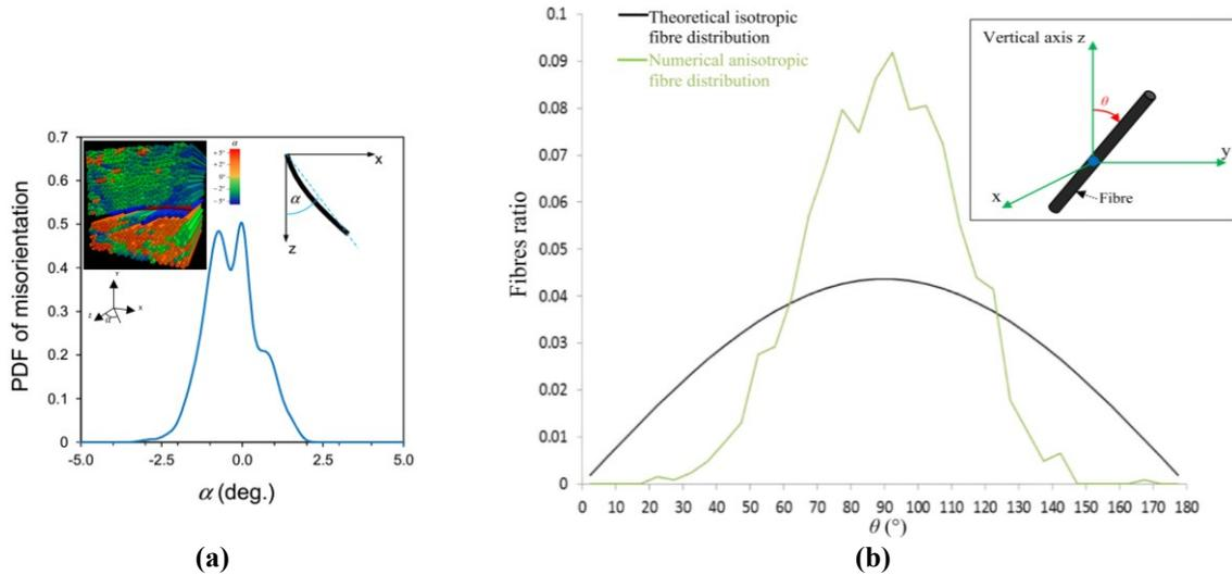
**Figure 2.9** Fiber orientation expressed by deflection angle. (a) PDF of fiber misalignment angle  $\alpha$  relative to the z-axis and the 3D CAD rendition of the segmented fibers with color scheme representing the  $\alpha$  (Czabaj et al., 2014). (b) Different fiber orientation distributions characterized by the angle between the fiber direction and the vertical Z-axis  $\theta$  (Chatti et al., 2020).
