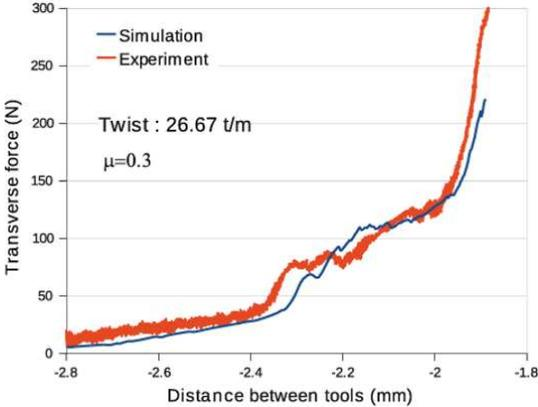
**Figure 3.17 Validate the simulation with experiment** (Moustaghfir et al., 2013).
