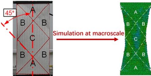
**Figure 1.6 Macroscale reinforcement modeling: Reinforcement is treated as a homogeneous material**
