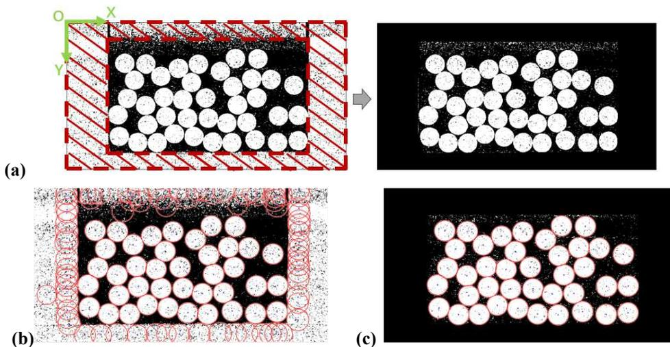
**Figure 5.3** Elimination of sample cassette (compaction plates/ channel). (a) Remove the compaction plates. (b), (c) With and eliminate the errors of the detection influenced by compaction plates, respectively.
