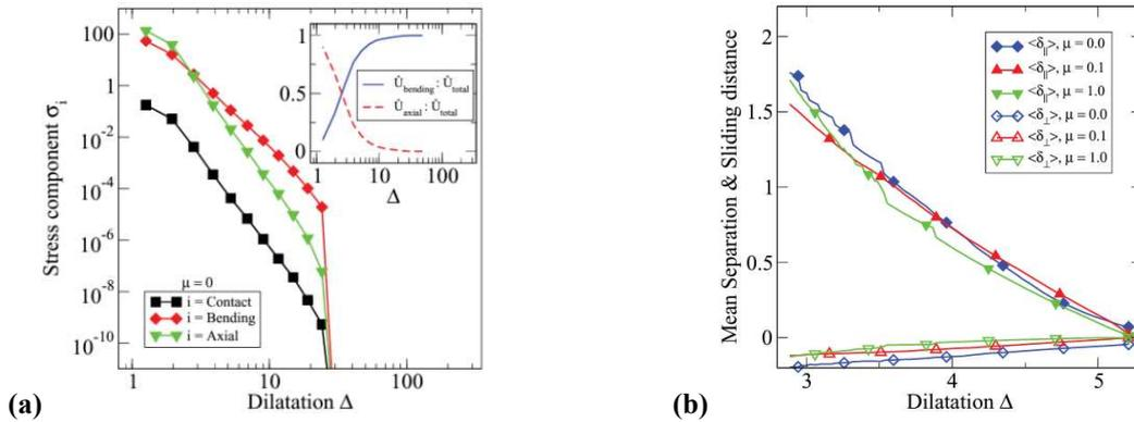
**Figure 3.8 Compaction of a 3D fibrous assembly. (a) Evolution of fiber contact, bending and tensile stresses as a function of  $\Delta$ . (b) Evolution of relative sliding and interpenetration distances between fibers for different friction coefficients  $\mu$  (Subramanian & Picu, 2011).**
