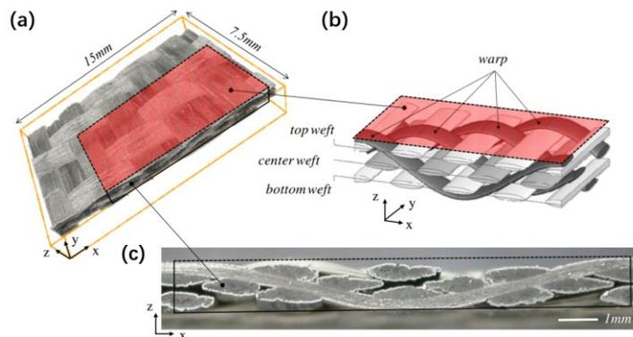
**Figure 3.1** The angle interlock architecture of the subject material: (a) 3D micro-CT image, (b) optical image of a cross-section along the warp direction, (c) idealized schematic of the unit cell (Rinaldi et al., 2012).
