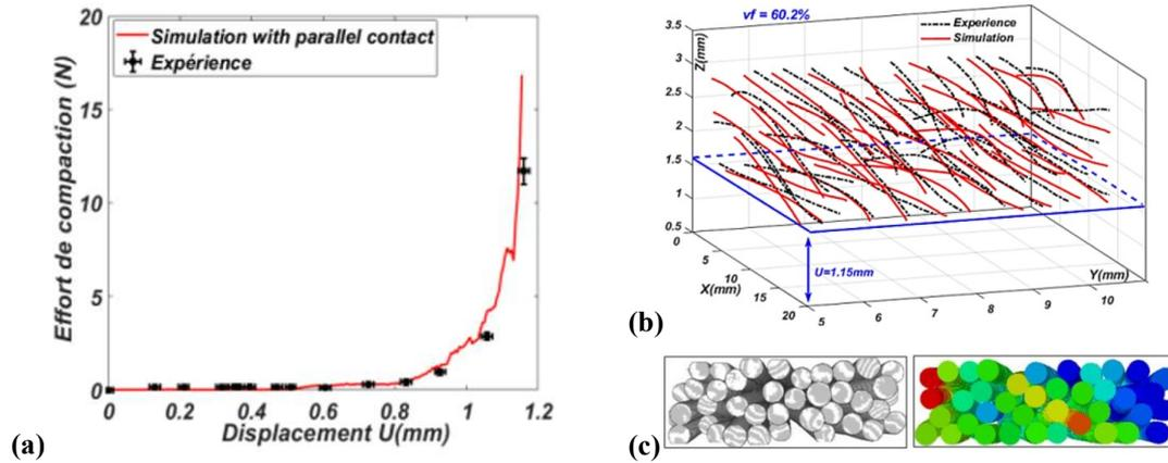
**Figure 1.10** The compaction simulation of 39 fibers. (a) The relationship between displacement of compaction plate and compaction force. (b) Centerline of fiber bundle at the last compaction step. (c) 3D geometry of fiber bundle at the last compaction step (Haji Oussama, 2018).
