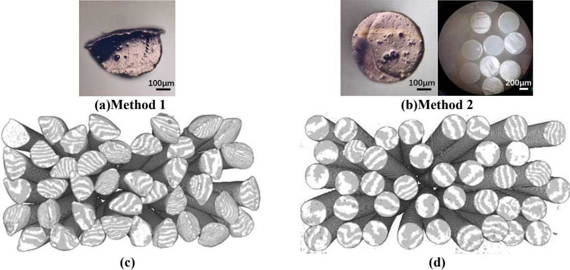
**Figure 4.1 Cross-section microscope images of single fibers for different methods of cutting fibers: (a) cutting method 1, (b) cutting method 2, tomography images of cross-sections at the end of fiber bundles: (c) sample obtained with cutting method 1, (d) sample obtained with cutting method 2.**
