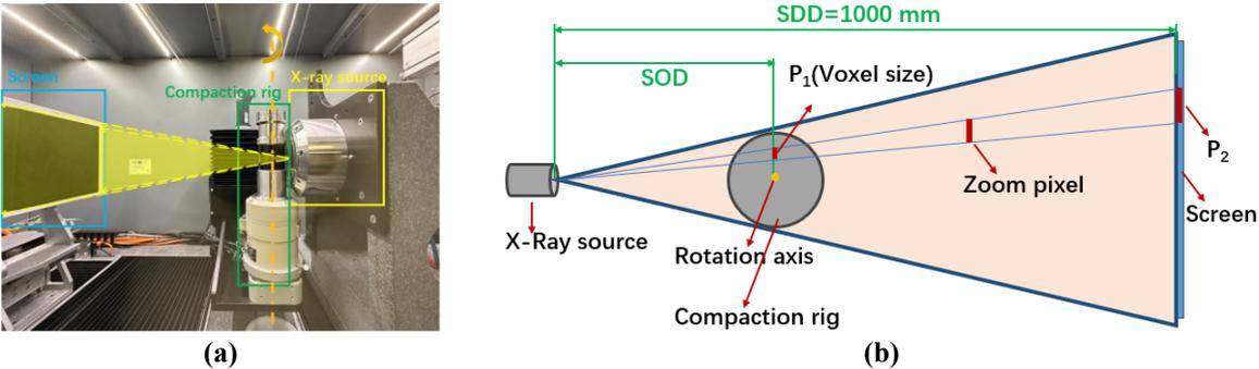
Figure 4.3 (a) X-ray tomography system, (b) Schematic diagram of the effect of sample location on spatial resolution (voxel size).
