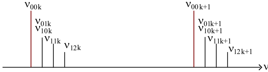
FIGURE 2.3: Spectrum of the transverse modes, where the indexes p, l of v_{plk} gives the number of nodes in the radial and angular profiles of the circular modes.
