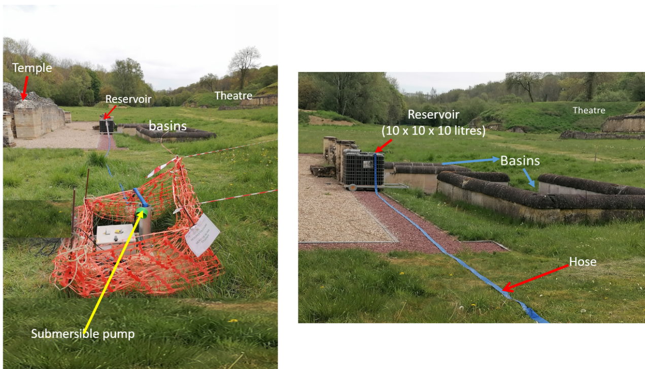
Figure 4.14: The picture on the left shows the materials used for the injection test experiment. The image on the right is the zoom of the item at the basins.
