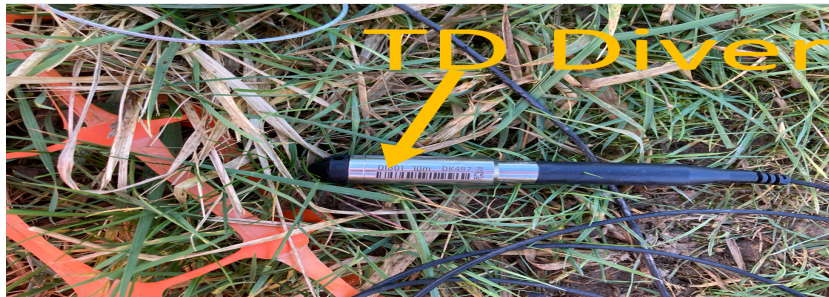
Figure 4.5: The TD-Diver installed at PzSa
