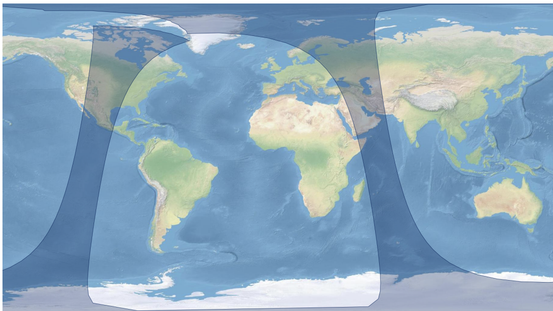
Figure 6 – An example of a IASI orbit footprint. Source: EUMETSAT Data Store https://data.eumetsat.int
