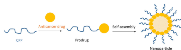
Figure 21 Scheme of the synthesis of prodrug nanoparticles.
