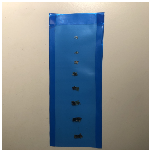
Figure 2.1 – The stages of mechanical exfoliation as seen through various flake sizes obtained.
