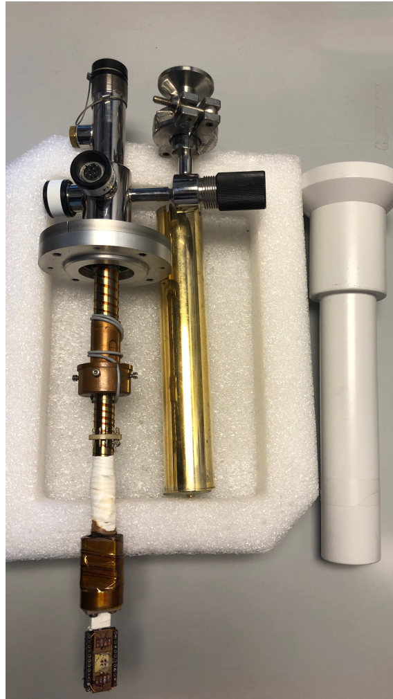
Figure 2.23 – The InSe device mounted within a cryostat, which doubles as a vacuum chamber
