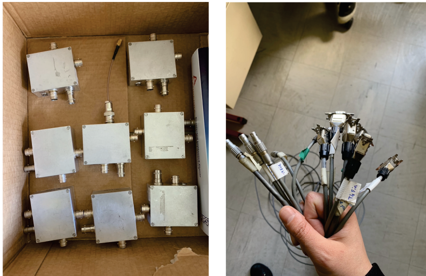
Figure 64: Photos of the 8 pre-amplifiers (left) and the low-voltage cables (right) supplied with the PIPS from the LPC.
