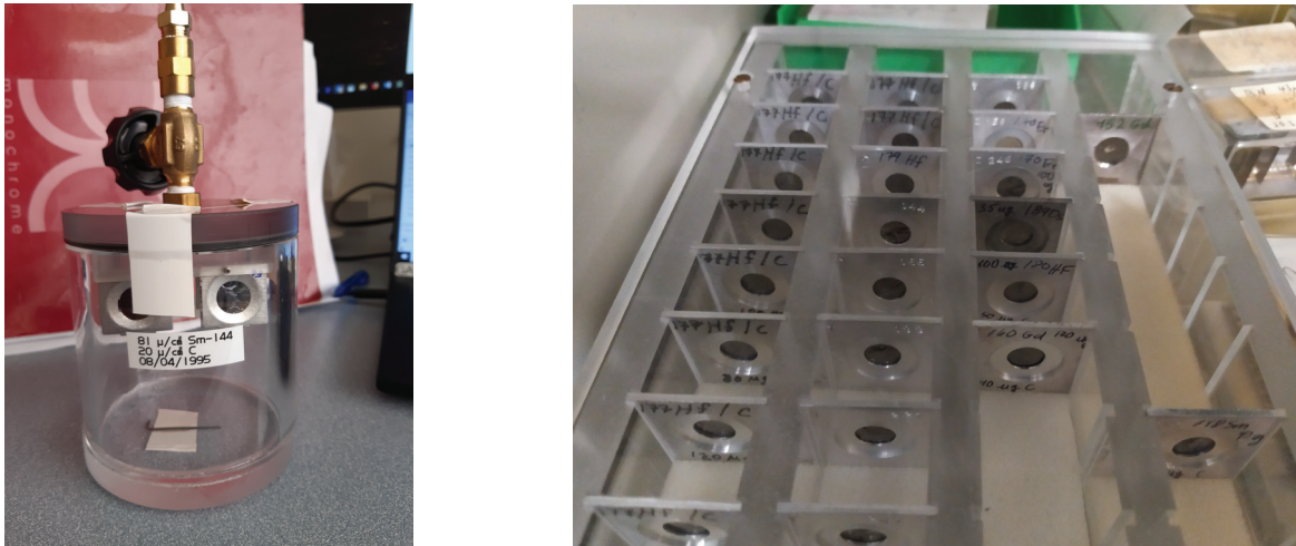
Figure 50: Pictures showcasing the two different storage methods of our targets. On the left, a vacuum reservoir contains two samarium targets from the Argonne National Laboratory, and on the right, a plastic box contains multiple hafnium targets sourced from the Technological Laboratory at the University of Munich.
