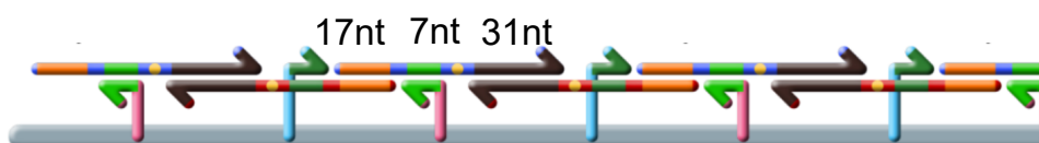
Figure 5.10: Assymetrical path design. The horizontal grey bar represents the top surface of the DNA origami. Vertical strands coming from this gray bar are "docking" staples. Yellow dots, represents the presence of a single-stranded flexible sequence TT allowing for turns.
