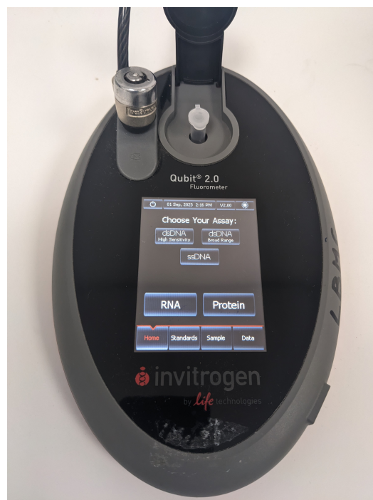
(b) Photos of the Qubit 2.0 with a tube inside and the lid open
