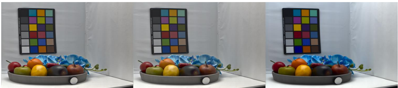
Figure 71, Sample images under N100 for Experiment 1: iCAM06 original (left), iCAM06 JzAzBz (center) and iCAM06 Guided filter (right)
