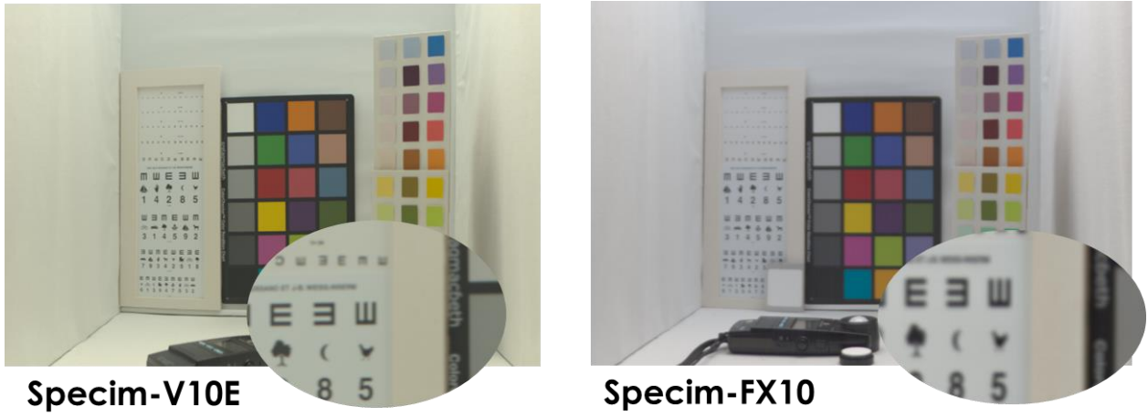
Figure 44, Color images treated with iCAM06 of hyperspectral data obtained from Specim V10E (left) and Specim FX10 (right); (Kuang et al, 2007)
