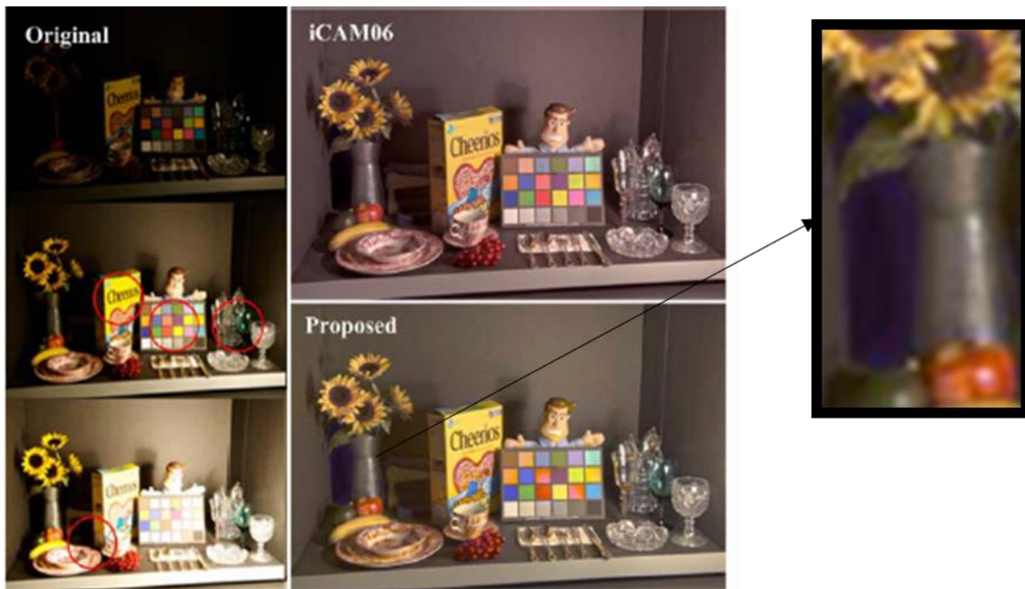
Figure 65, Blue artefacts due to saturation compensation (H.-G. Kim & Lee, 2013)
