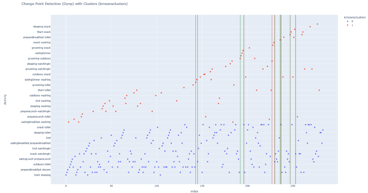
Figure 5.41 Ten change points detected with Dynamic Programming algorithm (red lines) and change points detected with Dynamic Programming and KMeans with 2 clusters (green lines) as scatter plot colored based on KMeans clusters. The length of each n-sequence of activities is 2 and Keras Tokenizer encoding technique was used.
