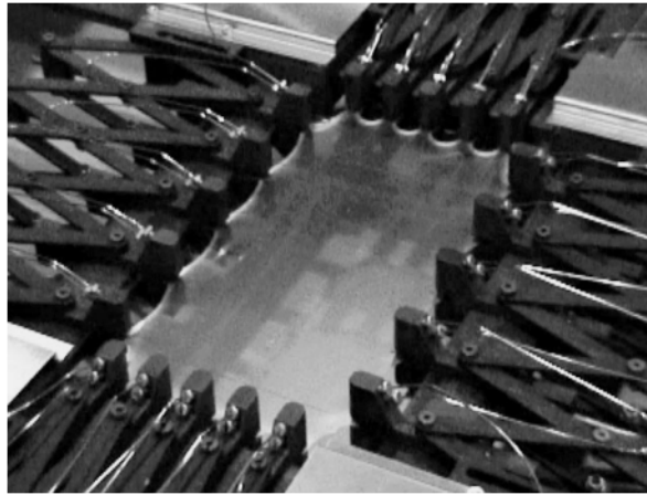
Figure 1.18: Bruckner biaxial stretching machine [60]
