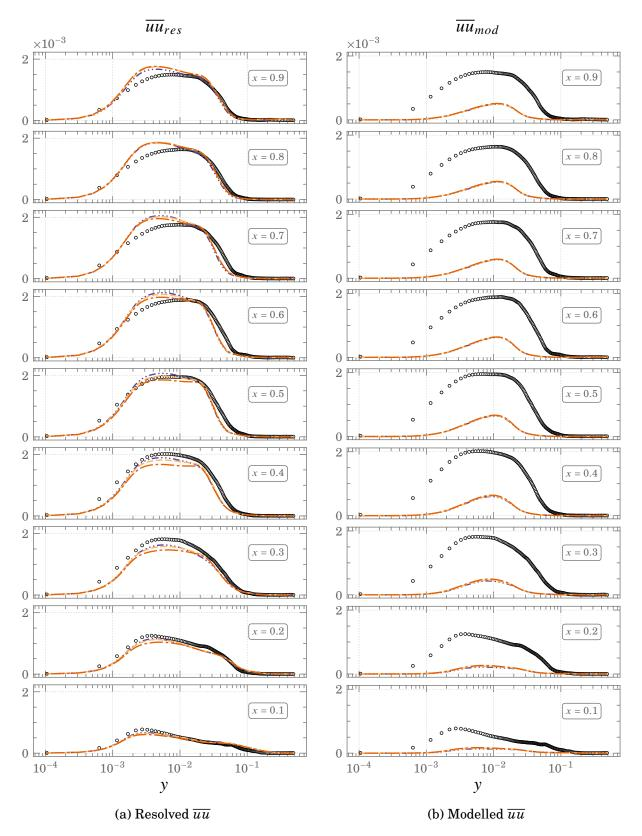
Figure 5.20.: Resolved and modelled contributions of  $\overline{uu}$  using the HTLES model for Square DHC at  $Ra=10^{11}$   $\circ \circ \circ DNS \quad --- FBE \quad ---- GGDH \quad -\cdots --- SGDH$
