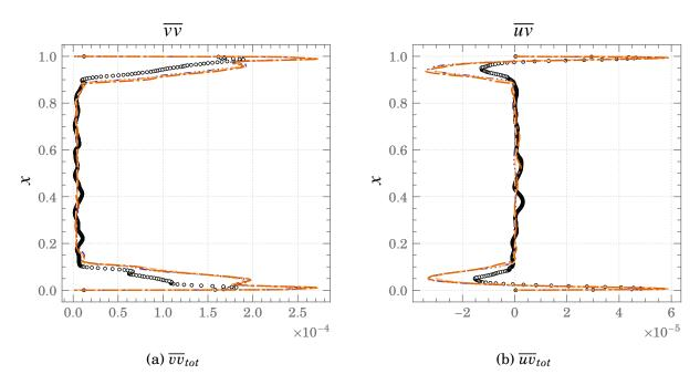
Figure A.11.: Comparisons of  $\overline{vv}_{tot}$  and  $\overline{uv}_{tot}$  profiles at the mid cavity (y=0.5) for Square DHC at  $Ra=10^{11}$   $\circ \circ \circ DNS \quad ---- 498 \times 80 \quad ---- 664 \times 80 \quad ---- 996 \times 100$
