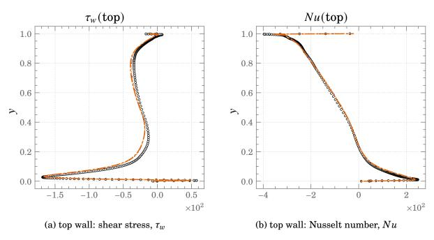
Figure A.20.: Comparisons of shear stress and Nusselt number profiles at the top wall for Square DHC at  $Ra=10^{11}$
