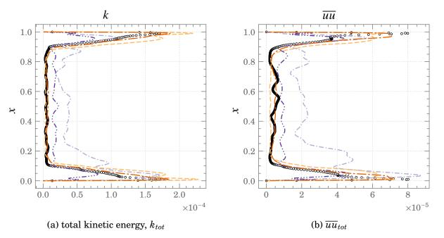
Figure 5.39.: Comparisons of total kinetic energy and  $\overline{uu}_{tot}$  profiles at the mid cavity (y=0.5) for Square DHC at  $Ra=10^{11}$   $\circ$   $\circ$   $\circ DNS$  ----- HTLES ---- LES ---- RANS-BL ----- RANS-KW
