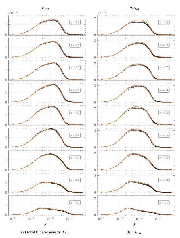
Figure A.14.: Comparisons of  $k_{tot}$  and  $\overline{uu}_{tot}$  profiles for Square DHC at  $Ra = 10^{11}$   $\circ$   $\circ$   $\circ$  DNS ---- SMAG ---- SMAG ---- WALE
