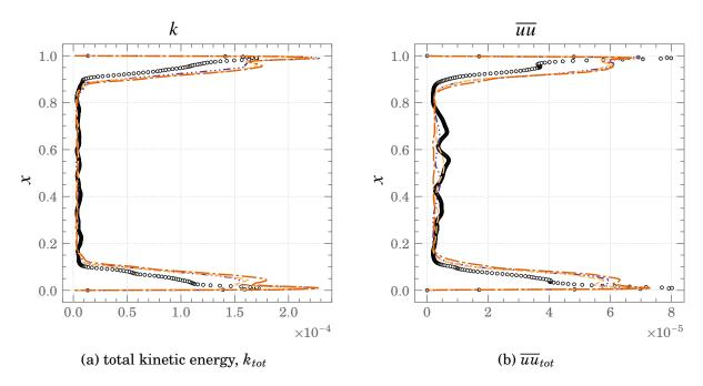
Figure A.22.: Comparisons of total kinetic energy and  $\overline{uu}_{tot}$  profiles at the mid cavity (y=0.5) for Square DHC at  $Ra=10^{11}$   $\circ$   $\circ$   $\circ$  DNS ---- Dyn-SMAG ---- WALE
