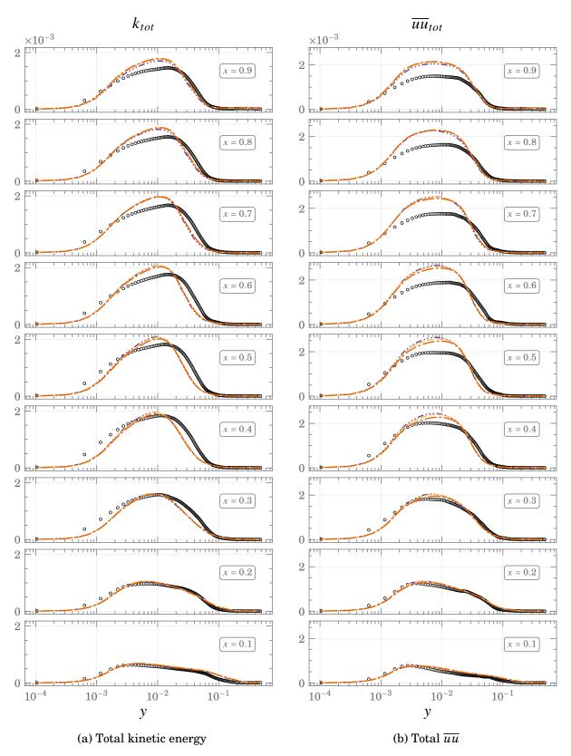
Figure 5.18.: Predictions of tital kinetic energy and total  $\overline{u}\overline{u}$  using the HTLES model for Square DHC at  $Ra = 10^{11}$
