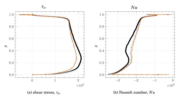
Figure A.7.: Comparisons of shear stress and Nusselt number profiles at the hot wall for Square DHC at  $Ra = 10^{11}$
