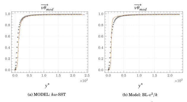
Figure 4.9.: Mean profiles of the Wall normal heat flux,  $\overrightarrow{v\theta}^+$   $\circ$   $\circ$   $\circ DNS$  --- GGDH --- SGDH
