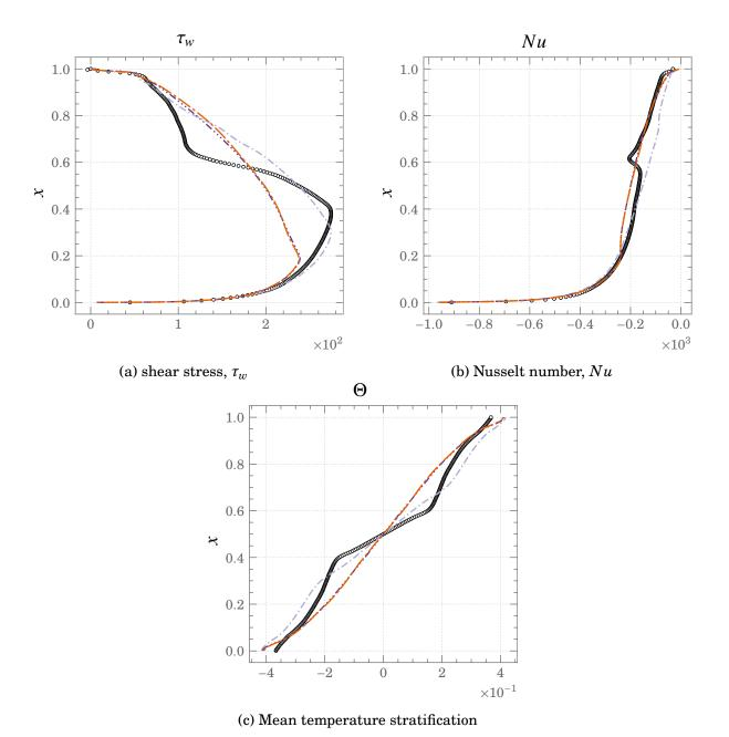
Figure B.1.: Comparisons of shear stress, Nusselt number, and temperature stratification profiles for Rectangular DHC at  $Ra=10^{11}$
