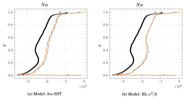
Figure 4.35.: Profiles of Nusselt number at the hot wall for  $Ra \times 10^{11}$   $\circ$   $\circ$   $\circ DNS$  ---- FBE ---- GGDH ---- SGDH
