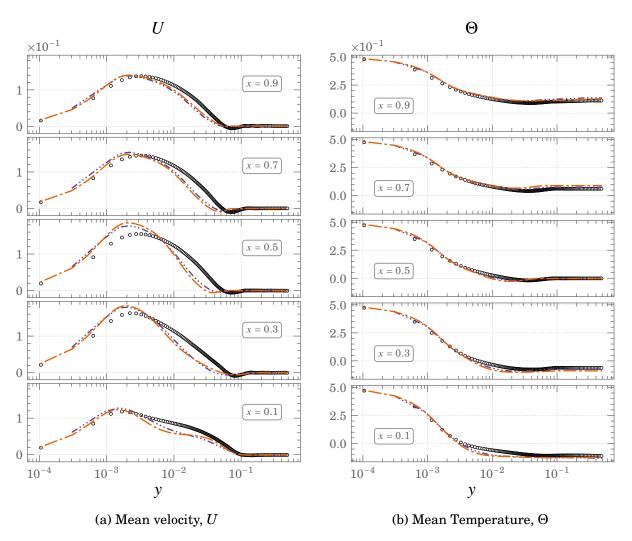
Figure 4.36.: Mean profiles of Velocity and Temperature for SGDH heat flux closure at  $Ra \times 10^{11}$  ° ° ° DNS ----  $G_{\omega}^{SST}$  -----  $G_{\omega}^{k\omega}$
