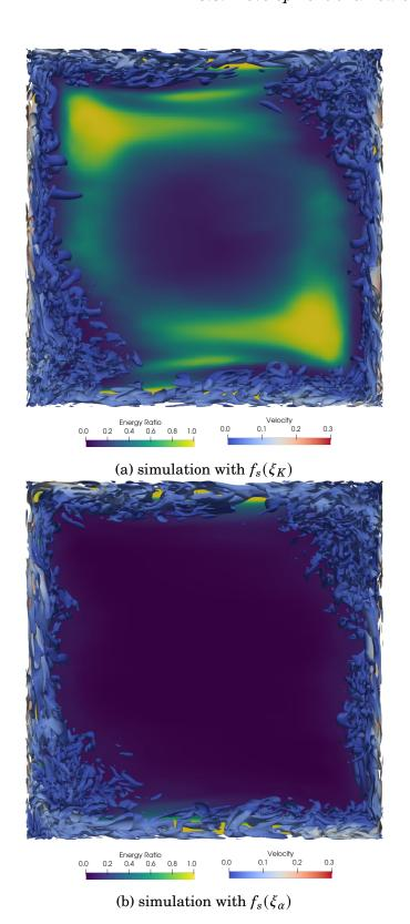
Figure 5.13.: Q-criterion of iso-contours at Q=0.1 with countour of the energy ratio in the background
