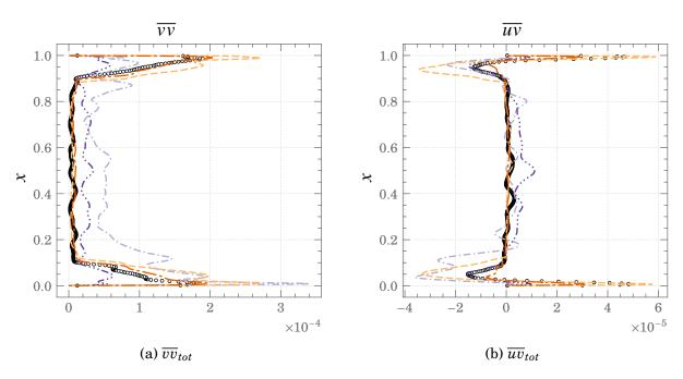
Figure 5.40.: Comparisons of  $\overline{vv}_{tot}$  and  $\overline{uv}_{tot}$  profiles at the mid cavity (y=0.5) for Square DHC at  $Ra = 10^{11}$  $\circ$   $\circ DNS$  ---- HTLES
