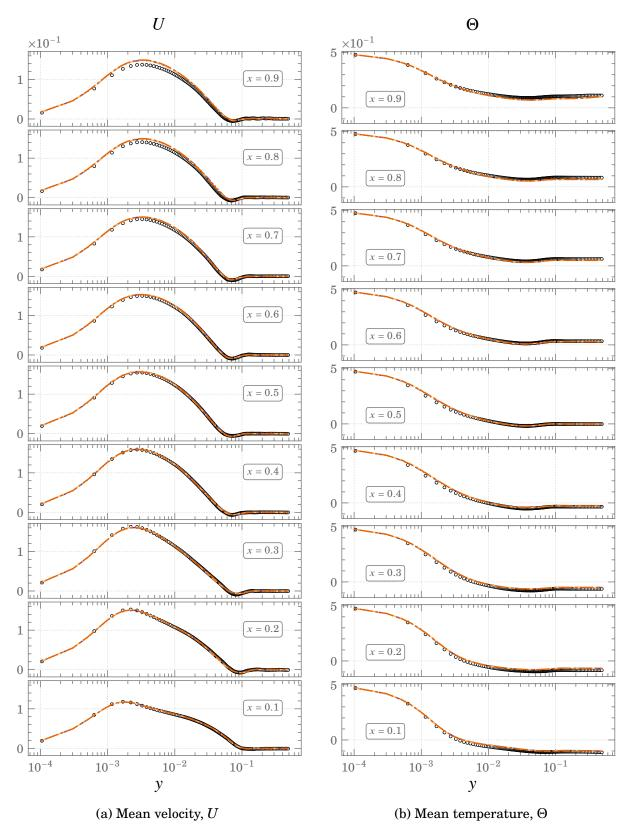
Figure A.13.: Comparisons of mean velocity and temperature profiles for Square DHC at  $Ra = 10^{11}$ ---- Dyn - SMAG
