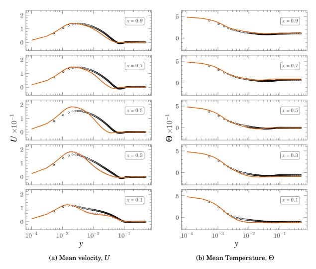
Figure 4.18.: Mean profiles of Velocity and Temperature for various meshes at  $Ra \times 10^{11}$   $\circ$   $\circ$   $\circ$   $\circ$  DNS  $\cdots$  249<sup>2</sup>  $\cdots$  332<sup>2</sup>  $\cdots$  415<sup>2</sup>  $\cdots$  498<sup>2</sup>
