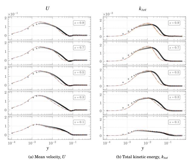
Figure 5.3.: Mean profiles of Velocity and total kinetic energy for various meshes at  $Ra \times 10^{11} \circ \circ \circ \mathrm{DNS} \longrightarrow 332^2 \times 40 \longrightarrow 332^2 \times 60 \longrightarrow 332^2 \times 80$
