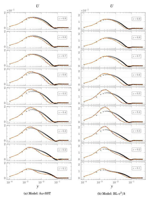
Figure 4.21.: Mean profiles of Velocity at  $Ra \times 10^{11}$  $\circ \circ \circ DNS \longrightarrow FBE \longrightarrow GGDH \longrightarrow SGDH$
