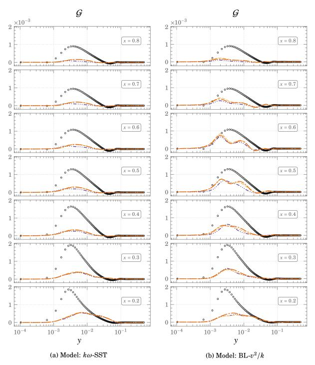
Figure 4.24.: Buoyancy production,  $\mathcal{G}$  for  $Ra \times 10^{11}$  $\circ \circ \circ DNS \longrightarrow FBE \longrightarrow GGDH \longrightarrow SGDH$
