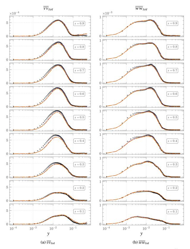
Figure A.15.: Comparisons of  $\overline{vv}_{tot}$  and  $\overline{ww}_{tot}$  profiles for Square DHC at  $Ra = 10^{11}$   $\circ$   $\circ$   $\circ DNS$  ---- Dyn - SMAG ---- WALE
