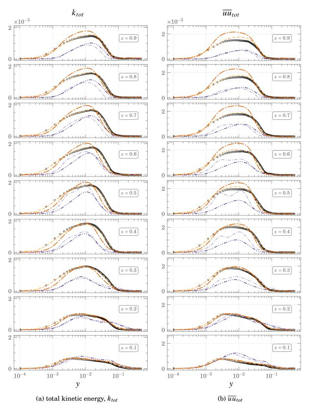
Figure 5.31.: Comparisons of  $k_{tot}$  and  $\overline{u}\overline{u}_{tot}$  profiles for Square DHC at  $Ra=10^{11}$   $\circ$   $\circ$   $\circ DNS$  ----- HTLES ---- LES ---- RANS-BL ----- RANS-KW
