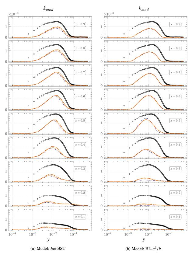
Figure 4.32.: Mean profiles of modelled turbulent kinetic energy,  $k_{mod}$ , at  $Ra \times 10^{11}$   $\circ$   $\circ$   $\circ DNS$  ---- FBE ---- GGDH ---- SGDH
