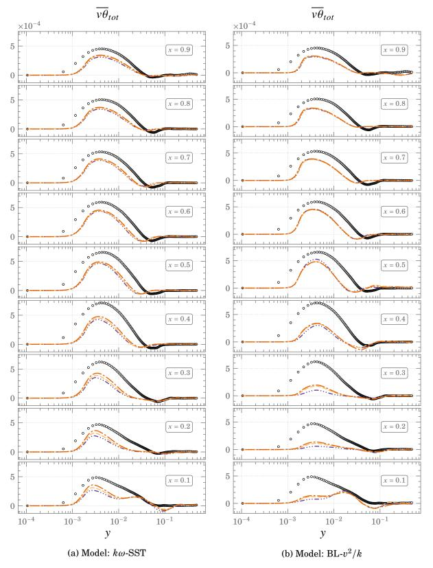
Figure 4.29.: Mean profiles of  $\overline{v\theta}$  at  $Ra \times 10^{11}$  $\circ \circ \circ DNS \longrightarrow FBE \longrightarrow GGDH \longrightarrow SGDH$
