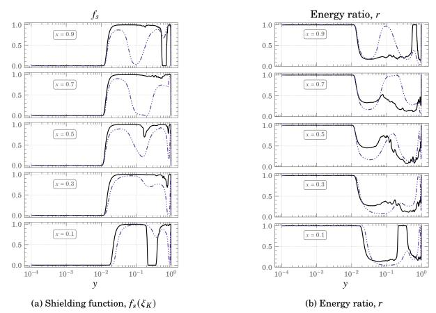
Figure 5.7.: Behaviour of the shielding function and its impact on the energy ratio in HTLES  $-\cdots--f_s(\xi_K)$ DNS
