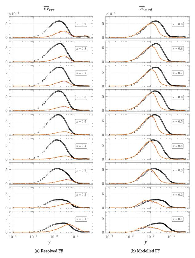
Figure 5.22.: Resolved and modelled contributions of  $\overline{vv}$  using the HTLES model for Square DHC at  $Ra=10^{11}$   $\circ \circ \circ DNS \quad ---- FBE \quad ---- GGDH \quad ----- SGDH$
