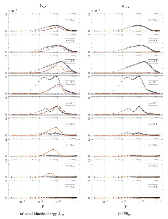
Figure B.3.: Comparisons of  $k_{tot}$  and  $k_{res}$  profiles for Rectangular DHC at  $Ra = 10^{11}$   $\circ \circ \circ DNS \longrightarrow HTLES \longrightarrow RANS - BL \longrightarrow RANS - KW$
