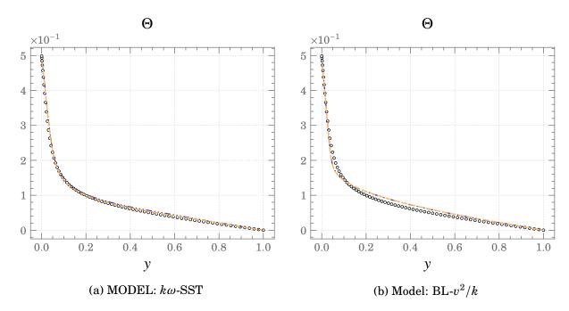
Figure 4.3.: Mean profiles of Temperature at  $Ra \approx 1.7 \times 10^7$  ( $Gr = 3 \times 10^6$ )  $\circ \circ \circ DNS \quad ---- GGDH \quad -\cdots - SGDH$
