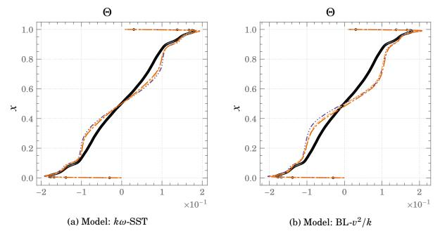
Figure 4.20.: Profiles of Temperature stratification at y = 0.5 for  $Ra \times 10^{11}$   $\circ$   $\circ$   $\circ DNS$  ---- FBE ---- GGDH ---- SGDH
