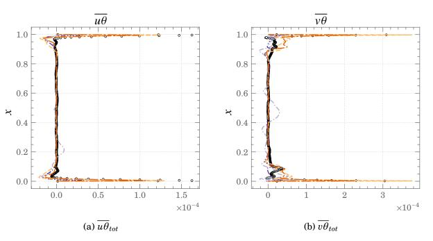
Figure 5.41.: Comparisons of  $\overline{u\theta}_{tot}$  and  $\overline{v\theta}_{tot}$  profiles at the mid cavity (y = 0.5) for Square DHC at  $Ra = 10^{11}$  $\circ \hspace{0.1cm} \circ \hspace{0.1cm} \circ \hspace{0.1cm} DNS \hspace{0.1cm} \stackrel{----}{----} HTLES \hspace{0.1cm} \stackrel{----}{-----} LES \hspace{0.1cm} \stackrel{-----}{-----} RANS - BL \hspace{0.1cm} \stackrel{-----}{-----} RANS - KW$
