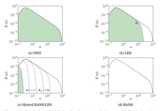
Figure 2.2.: Resolved and Modelled scales of various methods (green fill: Resolved scales)
