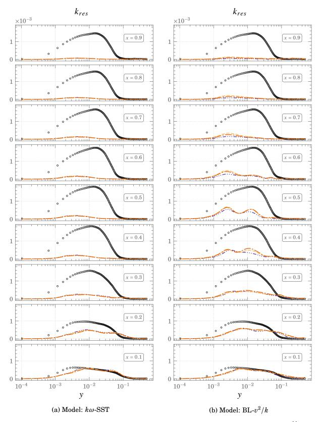
Figure 4.33.: Mean profiles of resolved urbulent kinetic energy,  $k_{res}$ , at  $Ra \times 10^{11}$   $\circ$   $\circ$   $\circ DNS$  ---- FBE ---- GGDH ---- SGDH
