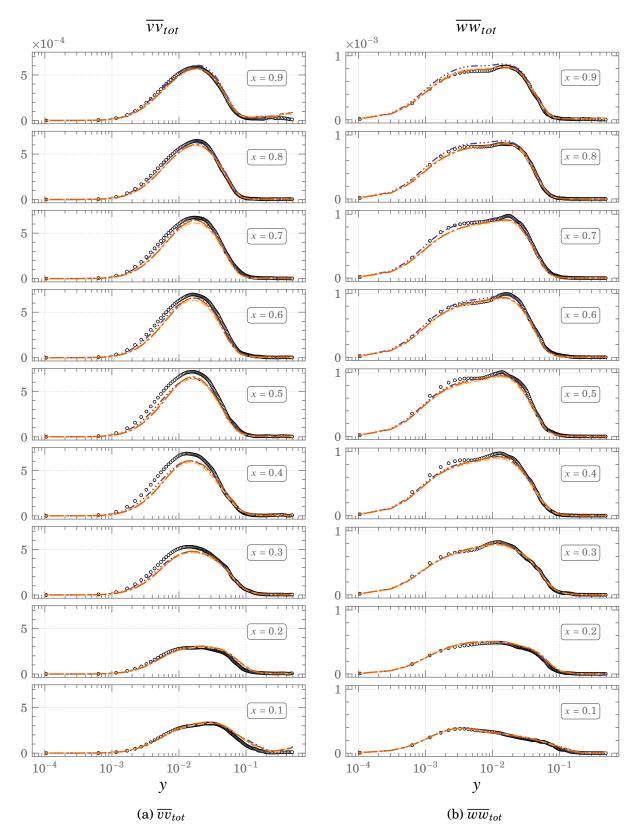
Figure A.3.: Comparisons of  $\overline{vv}_{tot}$  and  $\overline{ww}_{tot}$  profiles for Square DHC at  $Ra = 10^{11}$   $\circ$   $\circ$   $\circ DNS$  ----  $498 \times 80$  ----  $664 \times 80$  ----  $996 \times 100$
