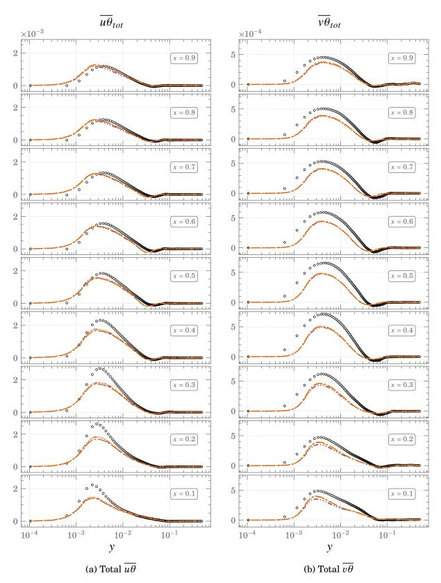
Figure 5.26.: Predictions of total  $\overline{u\theta}$  and total  $\overline{v\theta}$  using the HTLES model for Square DHC at  $Ra=10^{11}$   $\circ$   $\circ$   $\circ$  DNS ----- FBE ---- GGDH ----- SGDH
