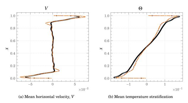
Figure A.9.: Comparisons of mean horizontal velocity and temperature strtification profiles at the mid cavity (y = 0.5) for Square DHC at  $Ra = 10^{11}$   $\circ \circ \circ DNS \longrightarrow 498 \times 80 \longrightarrow 664 \times 80 \longrightarrow 996 \times 100$
