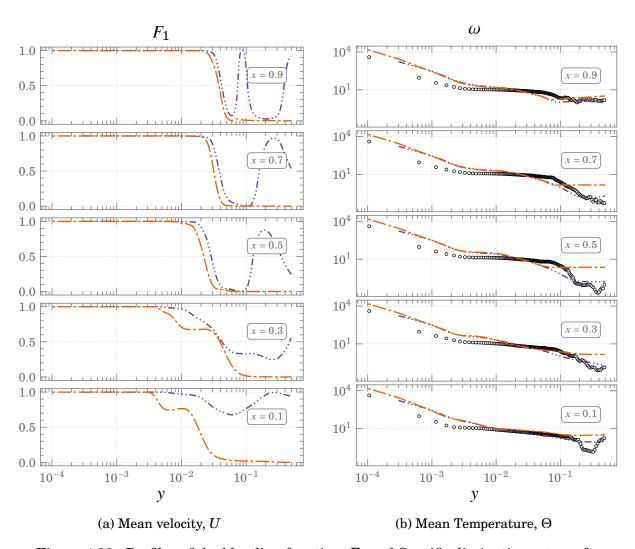
Figure 4.39.: Profiles of the blending function,  $F_1$  and Specific dissipation rate,  $\omega$  for SGDH heat flux closure at  $Ra \times 10^{11}$  ° ° ° DNS ----  $G_{\omega}^{SST}$  -----  $G_{\omega}^{k\omega}$
