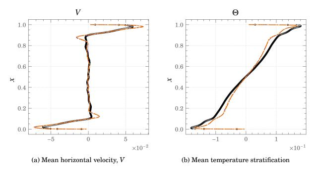
Figure A.21.: Comparisons of mean horizontal velocity and temperature strtification profiles at the mid cavity (y = 0.5) for Square DHC at  $Ra = 10^{11}$   $\circ$   $\circ$   $\circ$  DNS ---- Dyn - SMAG ---- WALE
