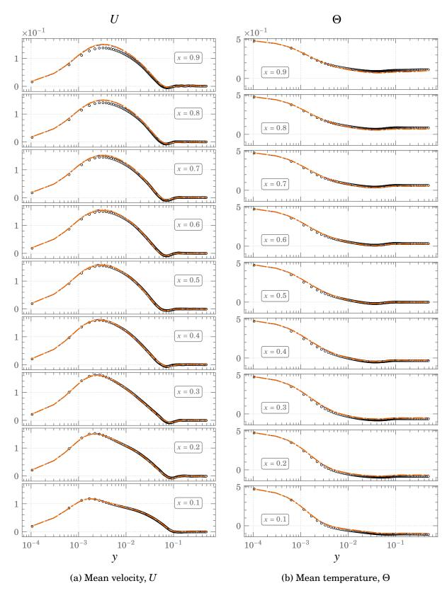
Figure A.1.: Comparisons of mean velocity and temperature profiles for Square DHC at  $Ra=10^{11}$   $\circ \circ \circ DNS \quad ---- 498\times 80 \quad ---- 664\times 80 \quad ---- 996\times 100$
