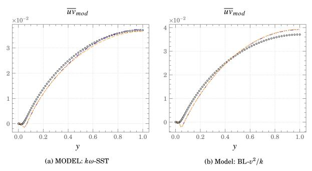
Figure 4.5.: Mean profiles of the turbulent shear stress,  $\overline{uv}$   $\circ$   $\circ$   $\circ$  ONS ---- GGDH ----- SGDH
