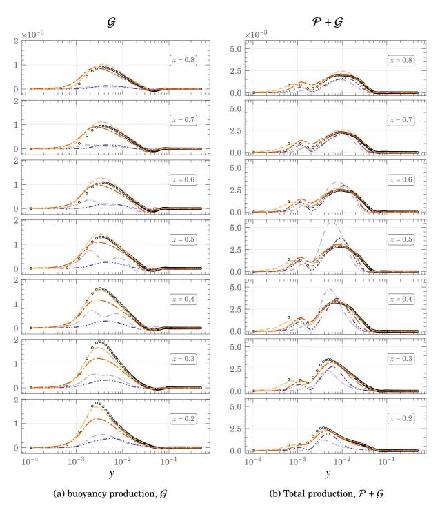
Figure 5.34.: Comparisons of buoyancy production,  $\mathcal{G}$ , and total production,  $\mathcal{P} + \mathcal{G}$ , profiles for Square DHC at  $Ra = 10^{11}$   $\circ \circ \circ DNS \longrightarrow HTLES \longrightarrow LES \longrightarrow RANS - BL \longrightarrow RANS - KW$
