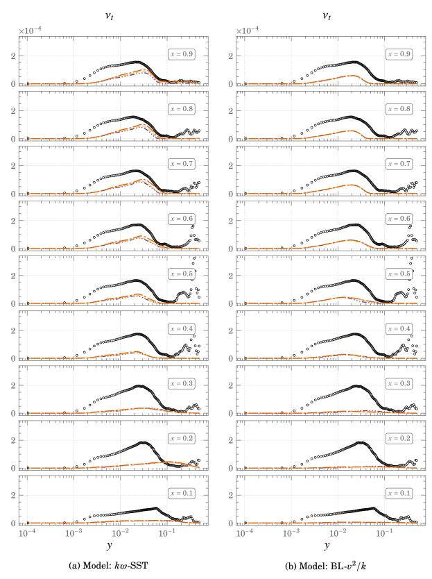
Figure 4.30.: Mean profiles of  $v_t$  at  $Ra \times 10^{11}$  $\circ \circ \circ DNS \longrightarrow FBE \longrightarrow GGDH \longrightarrow SGDH$
