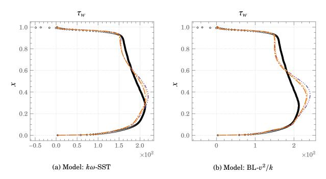
Figure 4.34.: Profiles of Wall shear stress,  $\tau_w$ , at the hot wall for  $Ra \times 10^{11}$   $\circ$   $\circ$   $\circ$  ONS ---- FBE ---- GGDH ----- SGDH
