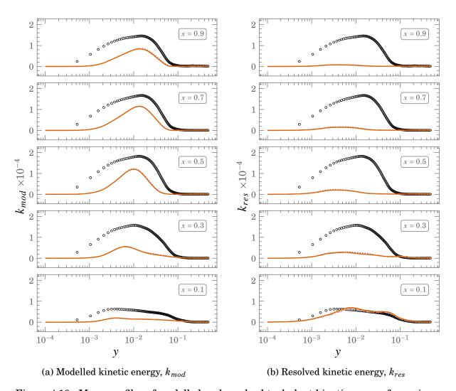
Figure 4.19.: Mean profiles of modelled and resolved turbulent kinetic energy for various meshes at  $Ra \times 10^{11}$   $\circ \circ \circ \circ \text{DNS} \qquad 249^2 \qquad ---- \qquad 415^2 \qquad 498^2$
