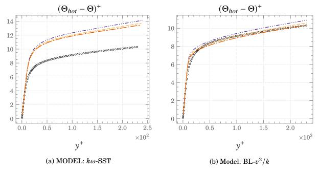
Figure 4.16.: Mean profiles of Temperature normalised with inner wall units at  $Ra \approx 1.7 \times 10^7 \ (Gr = 3 \times 10^6)$   $\circ \circ \circ DNS \longrightarrow FBE \longrightarrow GGDH \longrightarrow SGDH$
