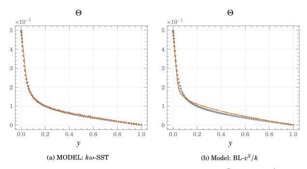
Figure 4.15.: Mean profiles of Temperature at  $Ra \approx 1.7 \times 10^7$  ( $Gr = 3 \times 10^6$ )  $\circ \circ \circ DNS \longrightarrow FBE \longrightarrow GGDH \longrightarrow SGDH$
