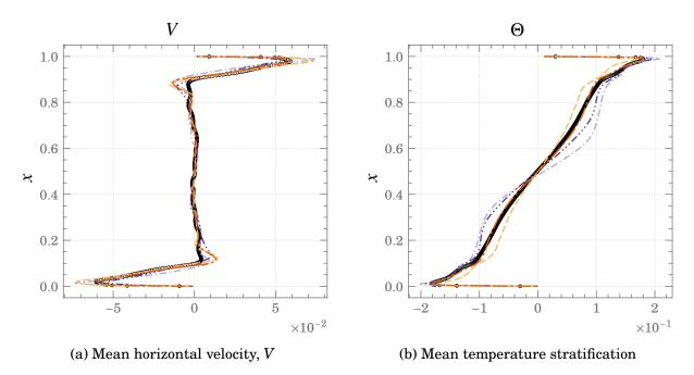
Figure 5.38.: Comparisons of mean horizontal velocity and temperature strtification profiles at the mid cavity (y = 0.5) for Square DHC at  $Ra = 10^{11}$   $\circ \circ \circ DNS \longrightarrow HTLES \longrightarrow LES \longrightarrow RANS - BL \longrightarrow RANS - KW$
