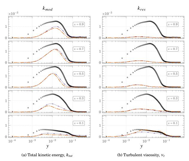
Figure 4.37.: Profiles of the modelled and resolved total kinetic energy for SGDH heat flux closure at  $Ra \times 10^{11}$  ° ° ° DNS ----  $G_{\omega}^{SST}$  -----  $G_{\omega}^{k\omega}$
