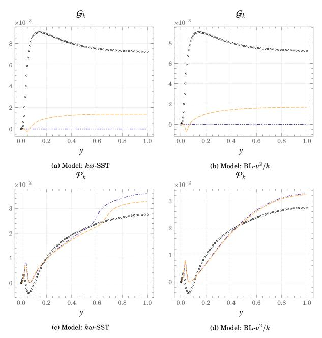
Figure 4.1.: Kinetic energy production,  $\mathcal{G}_k$  and  $\mathcal{P}_k$  at  $Ra \approx 1.7 \times 10^7$  ( $Gr = 3 \times 10^6$ )  $\circ \circ \circ DNS \quad ---- GGDH \quad -\cdots - SGDH$
