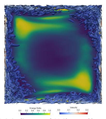
Figure 5.8.: Q-criterion of iso-contours at Q=0.1 with countour of the energy ratio in the background
