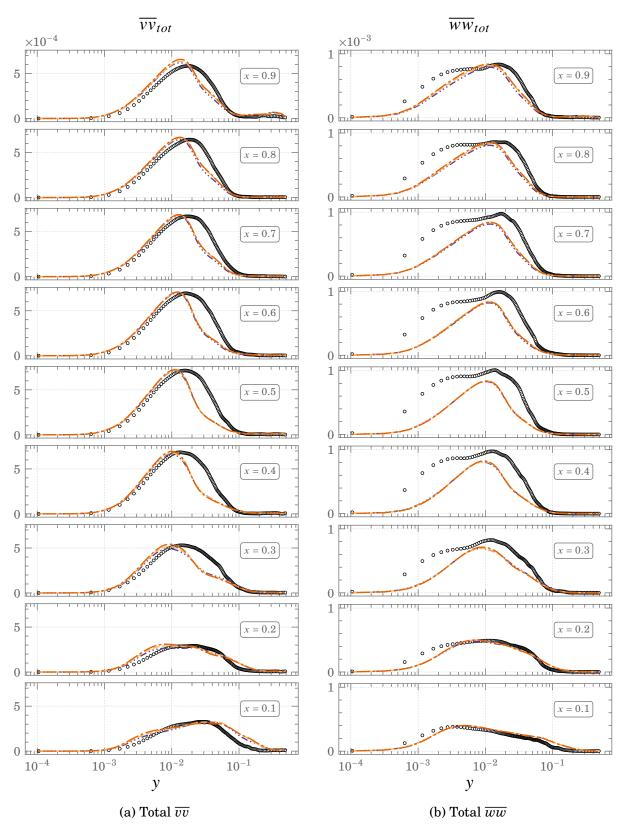
Figure 5.21.: Predictions of total  $\overline{vv}$  and total  $\overline{ww}$  using the HTLES model for Square DHC at  $Ra=10^{11}$   $\circ$   $\circ$   $\circ DNS$  ---- FBE ---- GGDH ----- SGDH
