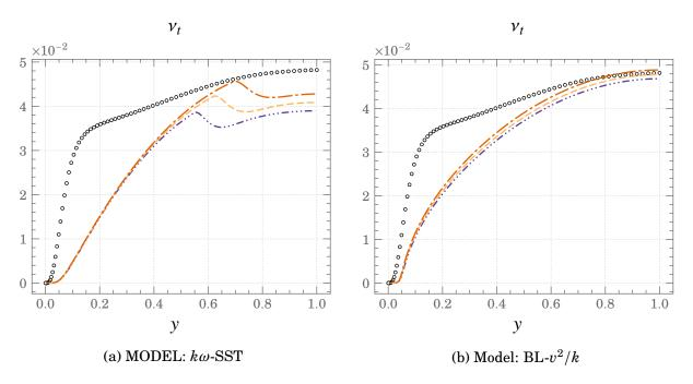
Figure 4.13.: Mean profiles of the turbulent viscosity,  $v_t$   $\circ \circ \circ DNS \longrightarrow FBE \longrightarrow GGDH \longrightarrow SGDH$
