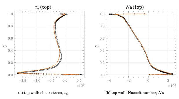
Figure A.8.: Comparisons of shear stress and Nusselt number profiles at the top wall for Square DHC at  $Ra = 10^{11}$
