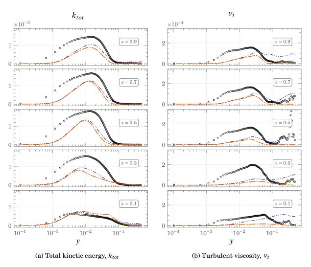
Figure 4.38.: Profiles of the total kinetic energy and turbulent viscosity for SGDH heat flux closure at  $Ra \times 10^{11}$  ° ° DNS ----  $G_{\omega}^{SST}$  -----  $G_{\omega}^{k\omega}$
