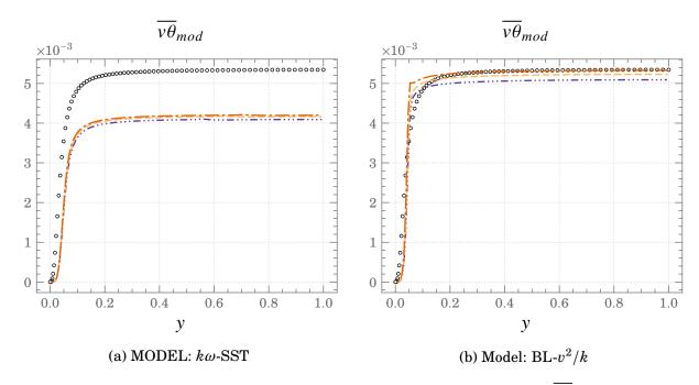
Figure 4.17.: Mean profiles of the Wall normal heat flux,  $\overline{v\theta}$   $\circ$   $\circ$   $\circ DNS$  ---- FBE ---- GGDH ----- SGDH
