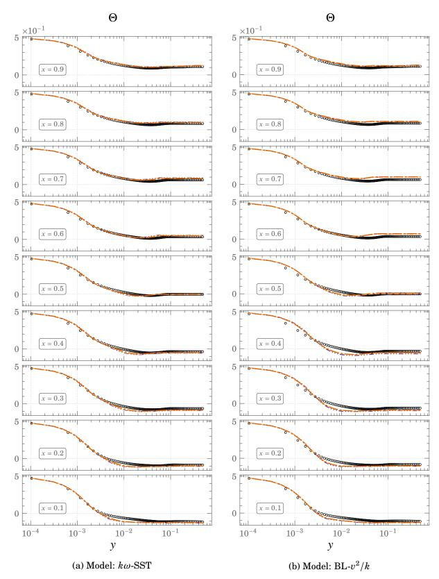
Figure 4.22.: Mean profiles of Temperature at  $Ra \times 10^{11}$   $\circ$   $\circ$   $\circ DNS$  ---- FBE ---- GGDH ---- SGDH
