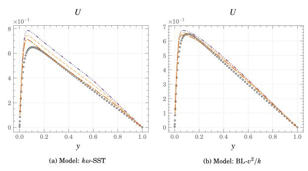
Figure 4.11.: Mean profiles of Velocity at  $Ra \approx 1.7 \times 10^7$  ( $Gr = 3 \times 10^6$ )  $\circ \circ \circ DNS \longrightarrow FBE \longrightarrow GGDH \longrightarrow SGDH$
