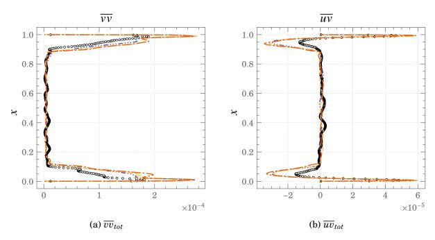
Figure A.23.: Comparisons of  $\overline{vv}_{tot}$  and  $\overline{uv}_{tot}$  profiles at the mid cavity (y=0.5) for Square DHC at  $Ra=10^{11}$   $\circ \circ \circ DNS \quad ---- Dyn-SMAG \quad ---- SMAG \quad ----- WALE$
