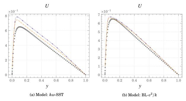
Figure 4.2.: Mean profiles of Velocity at  $Ra \approx 1.7 \times 10^7$  ( $Gr = 3 \times 10^6$ )  $\circ \circ ONS ---- GGDH ---- SGDH$
