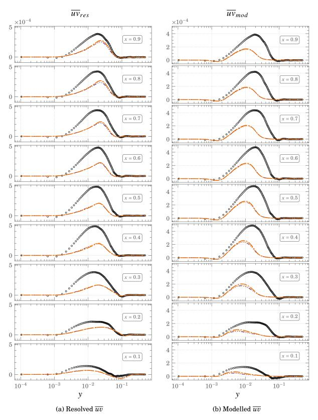
Figure 5.25.: Resolved and modelled contributions of  $\overline{uv}$  using the HTLES model for Square DHC at  $Ra=10^{11}$   $\circ \circ \circ DNS \quad ---- FBE \quad ---- GGDH \quad ----- SGDH$
