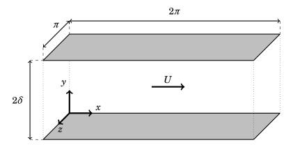
Figure 5.9.: Illustration of a forced channel flow
