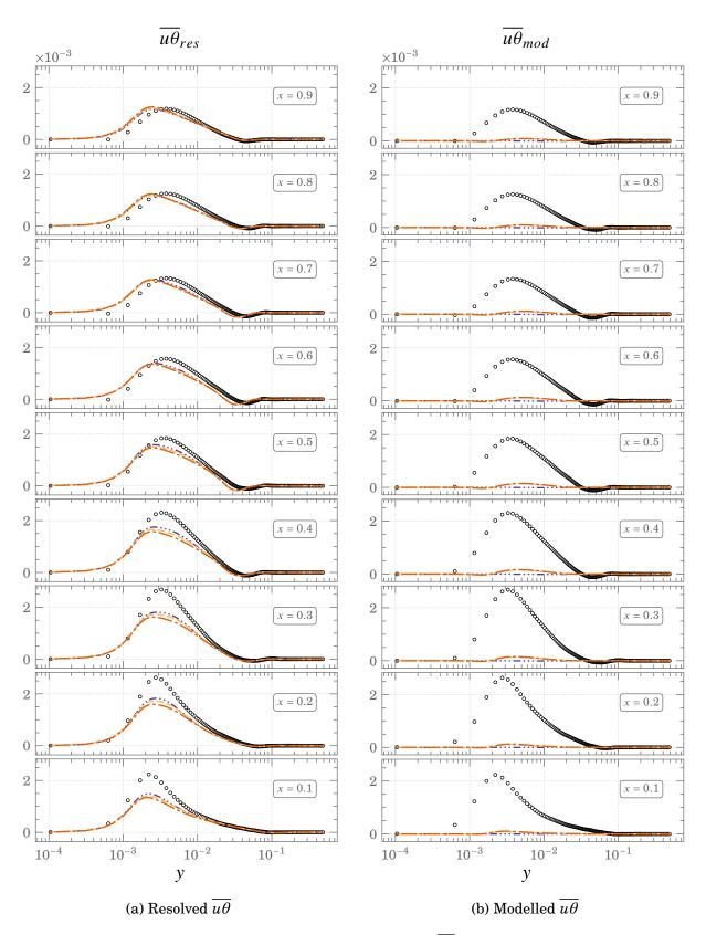
Figure 5.27.: Resolved and modelled contributions of  $\overline{ut}$  using the HTLES model for Square DHC at  $Ra = 10^{11}$   $\circ \circ \circ DNS \longrightarrow FBE \longrightarrow GGDH \longrightarrow SGDH$
