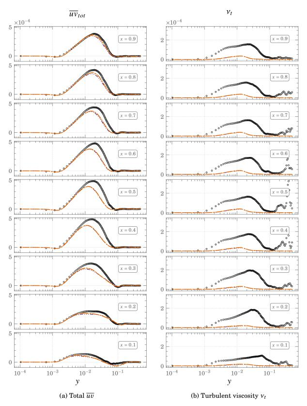
Figure 5.24.: Predictions of total shear stress,  $\overline{uv}$  and turbulent viscosity,  $v_t$  using the HTLES model for Square DHC at  $Ra=10^{11}$   $\circ \circ \circ DNS \longrightarrow FBE \longrightarrow GGDH \longrightarrow SGDH$
