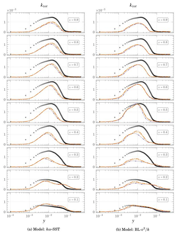
Figure 4.31.: Mean profiles of total turbulent kinetic energy,  $k_{tot}$ , at  $Ra \times 10^{11}$   $\circ$   $\circ$   $\circ DNS$  ---- FBE ---- GGDH ---- SGDH
