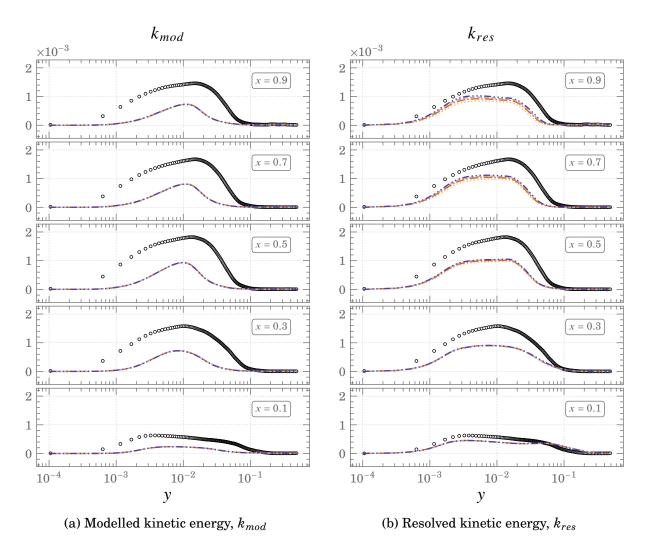
Figure 5.2.: Mean profiles of modelled and resolved turbulent kinetic energy for various meshes at  $Ra \times 10^{11}$   $\circ \circ \circ \text{DNS} \qquad 249^2 \qquad 332^2 \qquad 415^2 \qquad 498^2$
