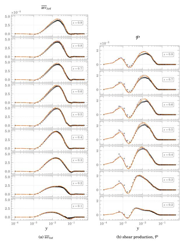
Figure A.4.: Comparisons of  $\overline{uv}_{tot}$  and shear production,  $\mathcal{P}$ , profiles for Square DHC at  $Ra=10^{11}$   $\circ \circ \circ DNS \quad ---- 498 \times 80 \quad ---- 664 \times 80 \quad ---- 996 \times 100$
