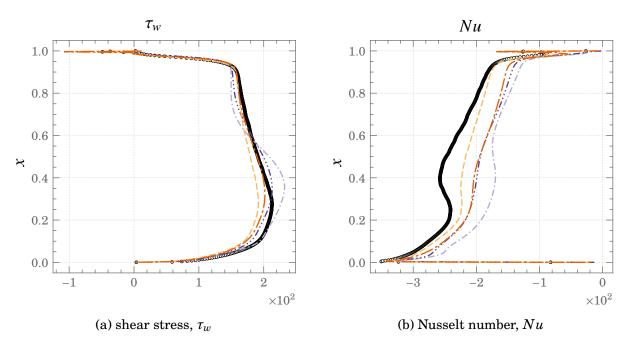
Figure 5.36.: Comparisons of shear stress and Nusselt number profiles at the hot wall for Square DHC at  $Ra = 10^{11}$
