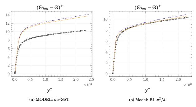
Figure 4.4.: Mean profiles of Temperature normalised with inner wall units at  $Ra \approx 1.7 \times 10^7 \ (Gr = 3 \times 10^6) \circ \circ ONS ----GGDH -----SGDH$
