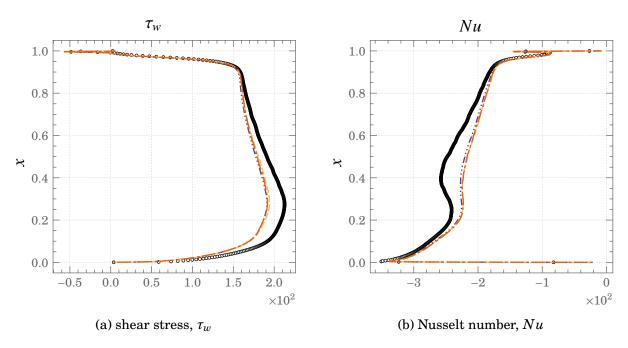
Figure A.19.: Comparisons of shear stress and Nusselt number profiles at the hot wall for Square DHC at  $Ra=10^{11}$   $\circ \circ \circ DNS \quad ---- Dyn-SMAG \quad ----- WALE$
