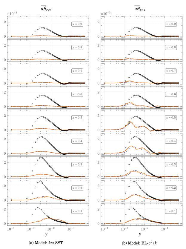
Figure 4.28.: Mean profiles of resolved  $\overline{u\theta}$  at  $Ra \times 10^{11}$   $\circ$   $\circ$   $\circ DNS$  ---- FBE ---- GGDH ---- SGDH
