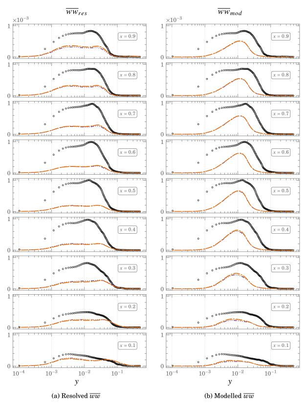
Figure 5.23.: Resolved and modelled contributions of  $\overline{ww}$  using the HTLES model for Square DHC at  $Ra=10^{11}$   $\circ \circ \circ DNS \quad ---- FBE \quad ---- GGDH \quad ----- SGDH$
