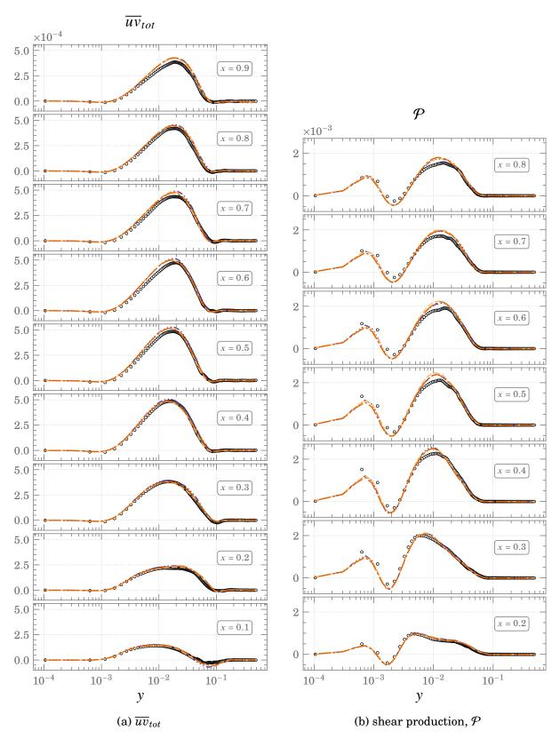
Figure A.16.: Comparisons of  $\overline{uv}_{tot}$  and shear production,  $\mathcal{P}$ , profiles for Square DHC at  $Ra = 10^{11}$   $\circ \circ \circ DNS \quad ---- Dyn - SMAG \quad ---- WALE$
