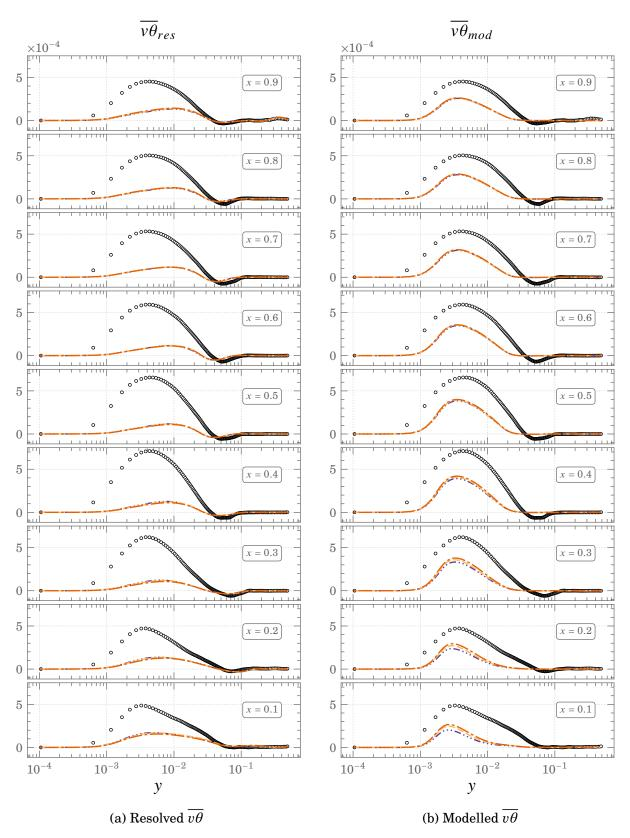
Figure 5.28.: Resolved and modelled contributions of  $\overline{v\theta}$  using the HTLES model for Square DHC at  $Ra=10^{11}$  of 0.000 of 0.
